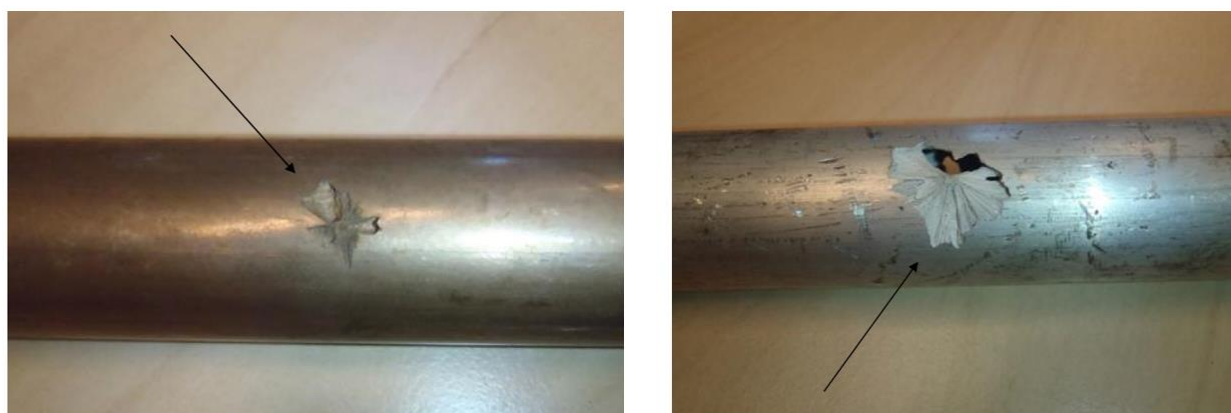
Figure 15. Test results, 750 bar, 10 cm stand-off of the perpendicular jet. Copper-Nickel on the left and Aluminum on the right. (DOW)
