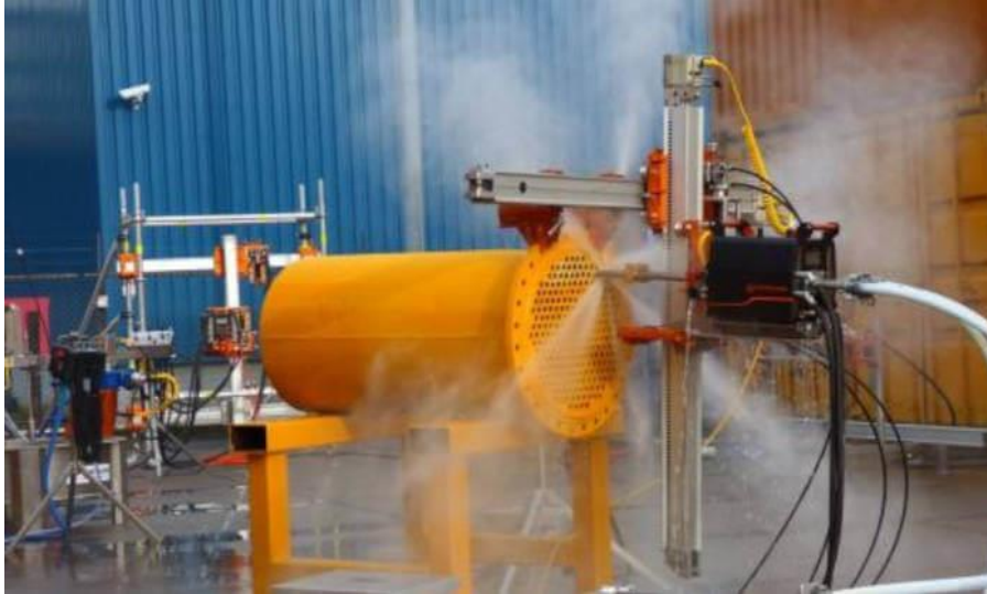
Figure 6. Automated heat exchanger tubes cleaner. (n.d.) Ax-system.com
