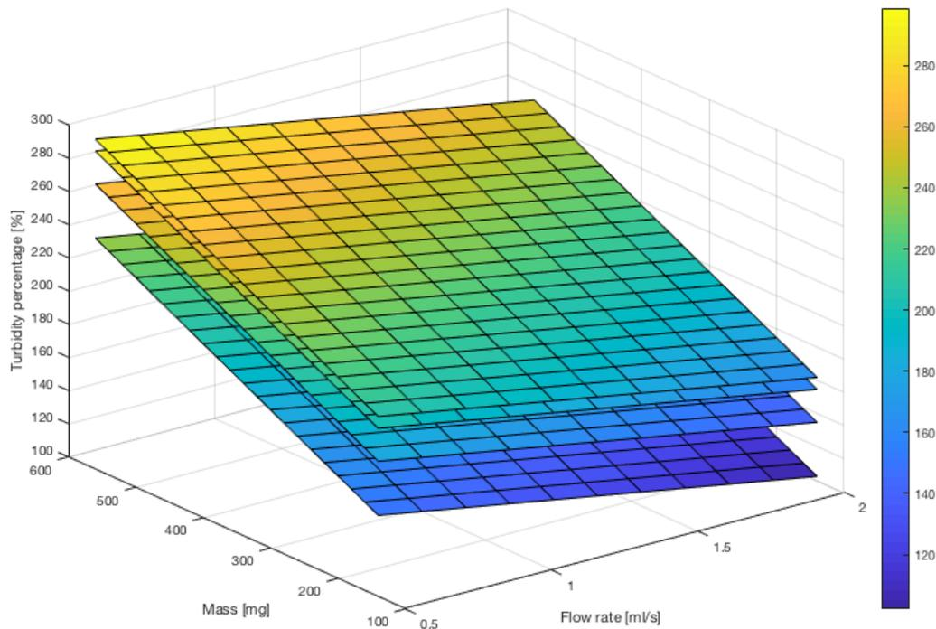
Figure 17 A 3-dimensional response surface plot for the concentrate model:  $f(Q, m, P) = -123 + -39Q + 75m + 494P - 192P^2$ . the layers represent the power outputs tested, the lowest layer being the lowest power (10W) and the upper layer being the highest (17.5W).
