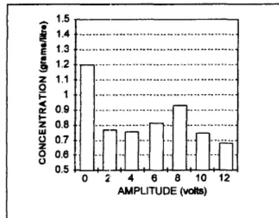
Figure 2 Separation concentration at applied voltages (Bekker, Meyer, Pretorius, & Van der Merwe, 1997)
