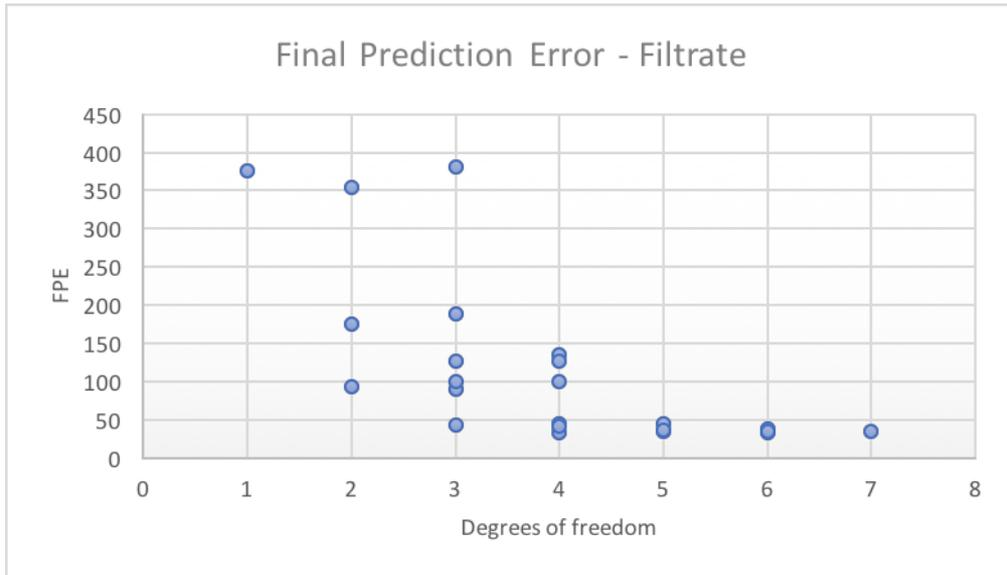
Figure 14 Final prediction error graph for the filtrate, the FPE value for each model is plotted against the degrees of freedom of that model.
