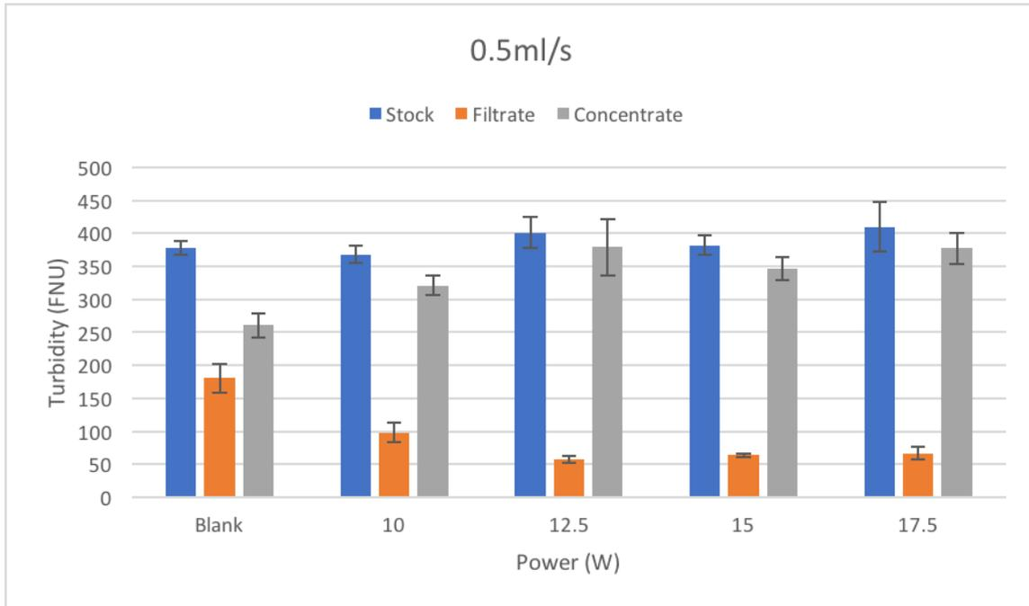
Figure 9 The effect of ultrasound on the turbidity of the filtrate and concentrate compared to that of the stock at varying power outputs at a flow of 0.5 ml/s. The error bars represent a 95% confidence interval.
