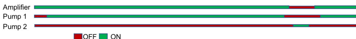
Figure 5 Time line of operation switching on and off times for the feed pump (pump 1) and the backwash pump (pump 2) and the amplifier in relation to each other (image courtesy of author).
