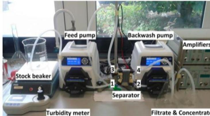
Figure 4 Particle separation unit set-up, equipment is labelled in the picture, numbered inlets/outlets is (1) inlet, (2) backwash, (3) air-fluid damper, (4) filtration outlet (Capon, 2014)
