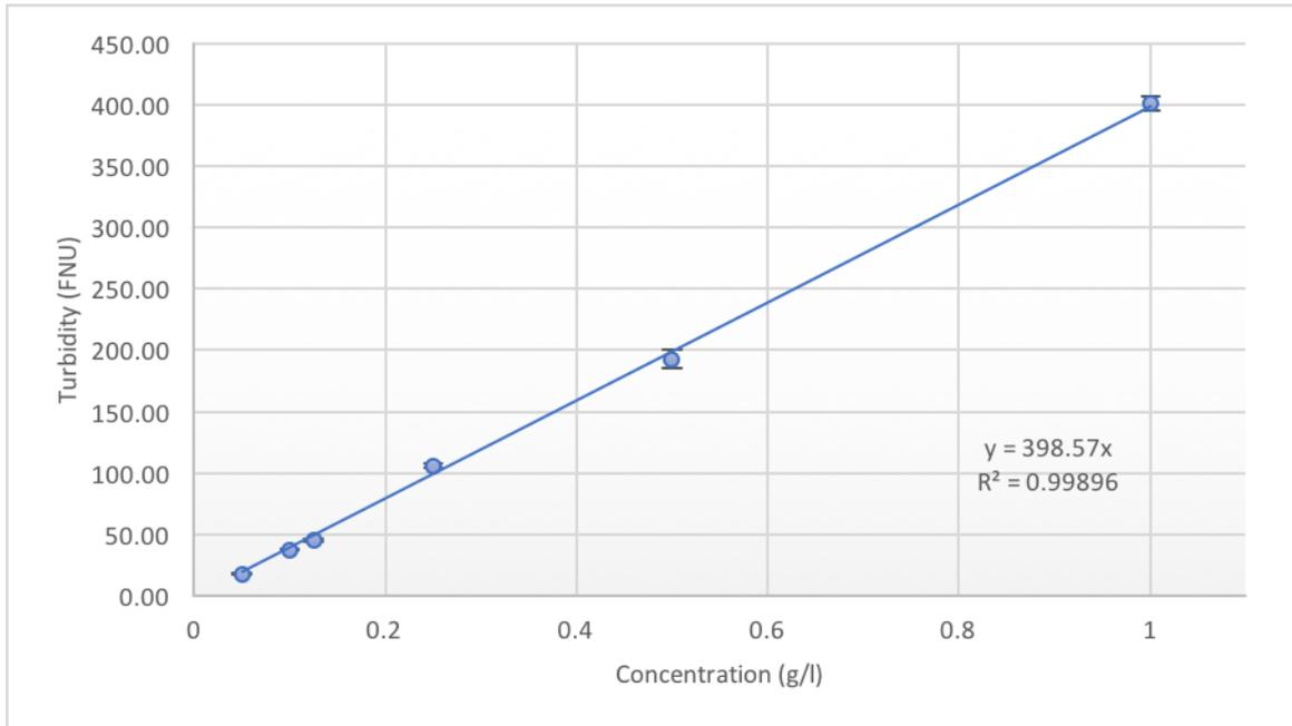
Figure 7 Graph displaying the relationship between turbidity and concentration. The error bars show the standard error per point, and the line equation ( $y = 398.57x$ ) and fit of the line ( $R^2 = 0.99896$ ) are also displayed.
