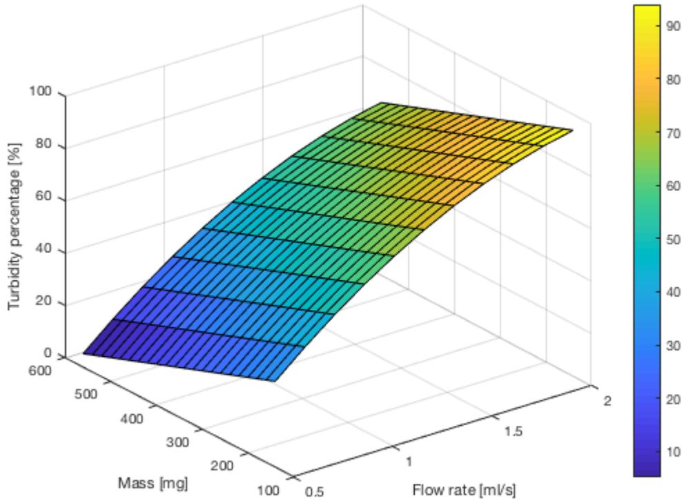
Figure 16 A 3-dimensional response surface plot for the filtrate model:  $f(Q, m) = 4 + 106Q - 23m - 28Q^2$ .
