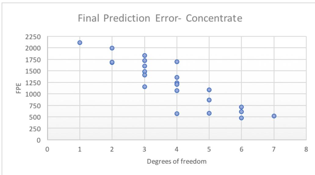
Figure 15 Final prediction error graph for the concentrate, the FPE value for each model is plotted against the degrees of freedom of that model.
