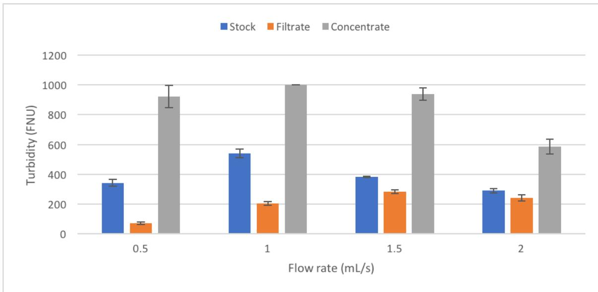
Figure 13 The effect of flow rate on the turbidity of the filtrate and concentrate compared to that of the stock at constant power output of 12.5W with a processed starch mass of 0.42g for all flow rates.
