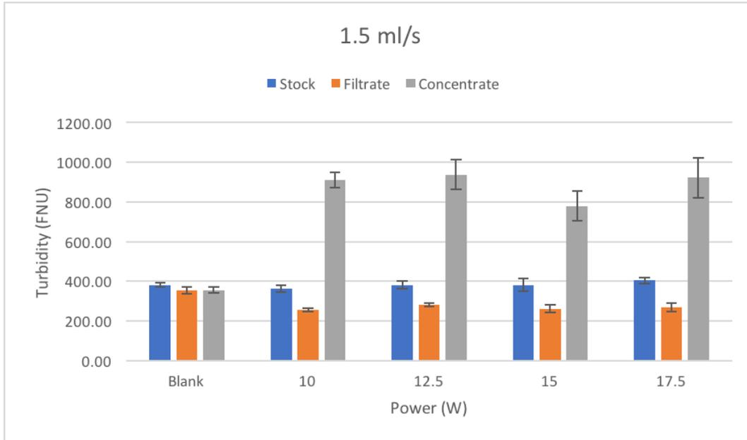
Figure 11 The effect of ultrasound on the turbidity of the filtrate and concentrate compared to that of the stock at varying power outputs at a flow of 1.5 ml/s.
