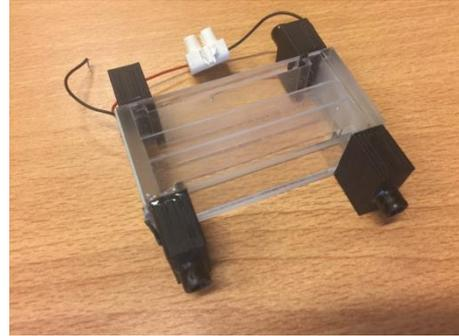
Figure 3 Separator designed by H.J. Cappon. wiring is for connection of transducers and black fixings are inlets and outlets for the fluid. (Image courtesy of author,2017)
