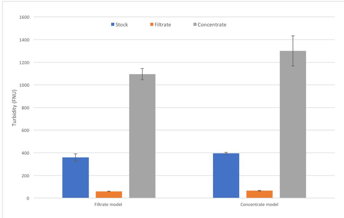
**Figure 18** Validation runs for optimal settings for each of the filtrate model, with setting of 0.5 ml/s, 12.5W of power and 560mg of processed starch mass, and the concentrate model with settings of 0.5ml/s, 17.5W and 560mg of processed starch.
