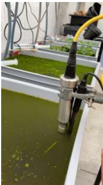
Figure 8- Side view of HACH HQ40d while measuring pH, dissolved oxygen, and temperature. (Elzinga, 2021)
