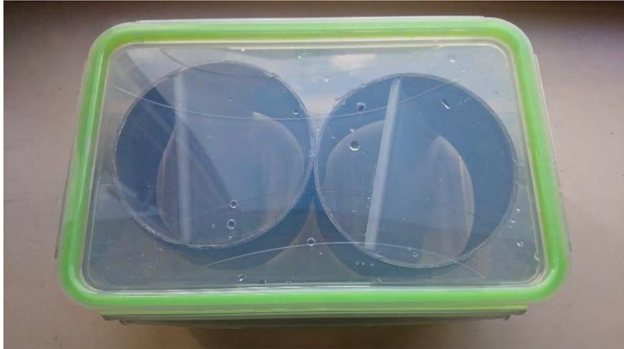
Figure 37. Preservation system for small panels under water. A rubber seal watertight container staked with two 90 mm PVC pipes.
