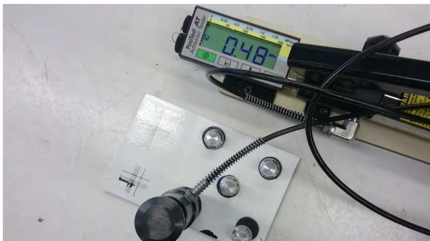
Figure 39. DeFelsko Positest AT-M Pull-Off Adhesion tester in action
