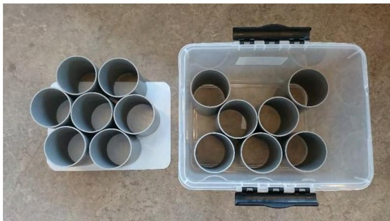
*Figure 36. Preservation of full-sized panels made out of 180 mm PVC DN 125 piping. Stories were separated sing a thin foamed polystyrene sheet. A lid was used to close the container.*
