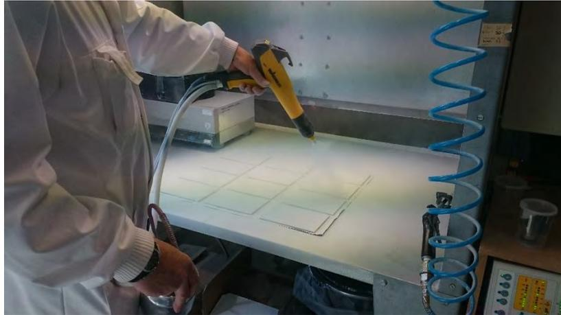
Figure 5. Manual application of a powder coating
