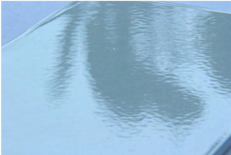
*Figure 44. Close up visual appearance of the polyester UV cured coating system applied on  $N_2$  plasma treated surface - treatment time 60 s*
