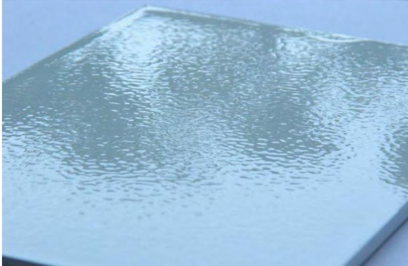
*Figure 42. Close up visual appearance of the hybrid coating system applied on  $N_2$  plasma treated surface - treatment time 60 s*
