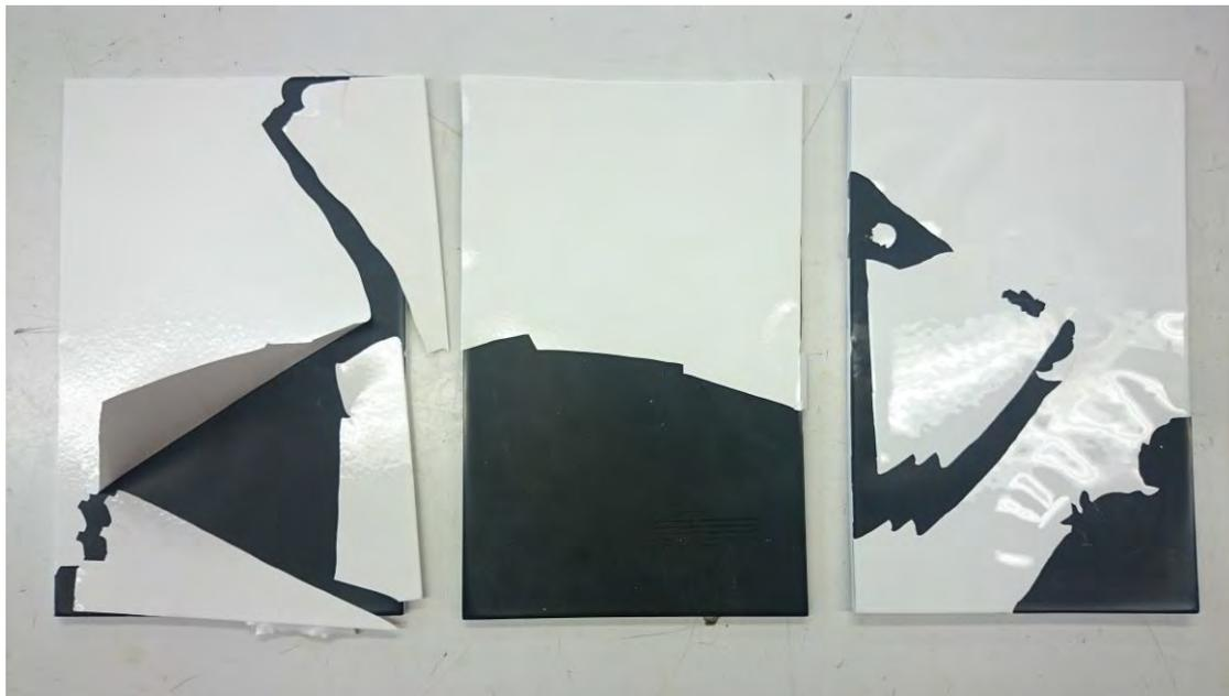
*Figure 21. Total absence of adhesion on untreated panel. Left to right: polyamide coating, hybrid coating and polyester UV coating system*
