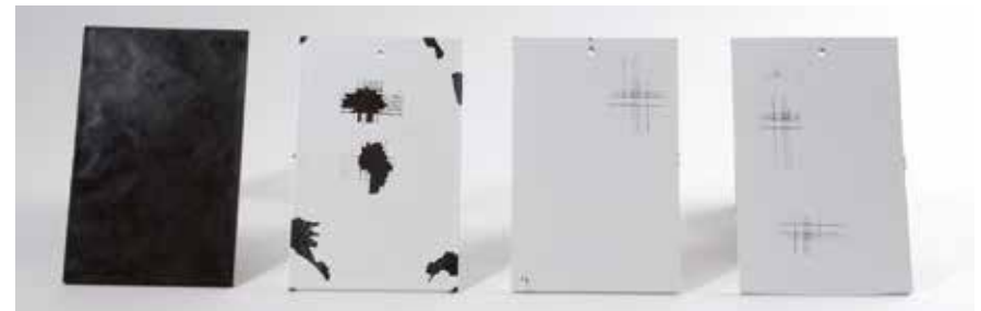
Project "Recycling of Polymeric Materials": Adhesion and Gitterschnitt tests on powder-coated PP test panels.
