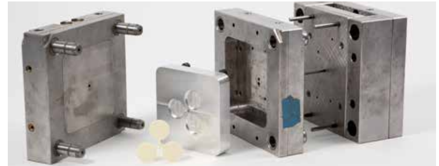
Quick mould change system for injection Moulding.
