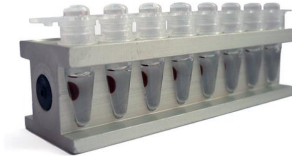
Figure 13: Magnetic rack with the samples: solid phase with the magnetic beads are attracted to the magnetic rack – they are visible as brown spots. The liquid phase can be removed without disturbing the magnetic beads. (18)
