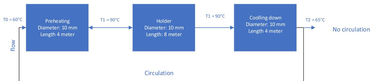
Fig. 1. Schematic overview of the used simulation model with the options for no-circulation and circulation.
