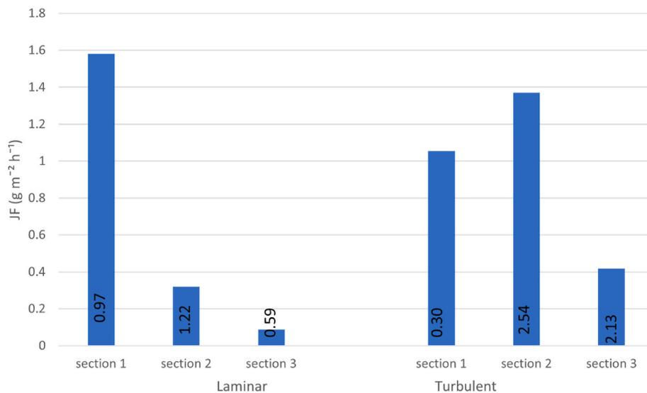
Fig. 4. Comparison between calculated fouling rates in different sections with turbulent and laminar flow (inlet 60 °C, holding 90 °C, outlet 60 °C) near the surface with  $Re = 2300$ . In the bars the average amount of denatured  $\beta$ -lactoglobulin is shown (g/l).
