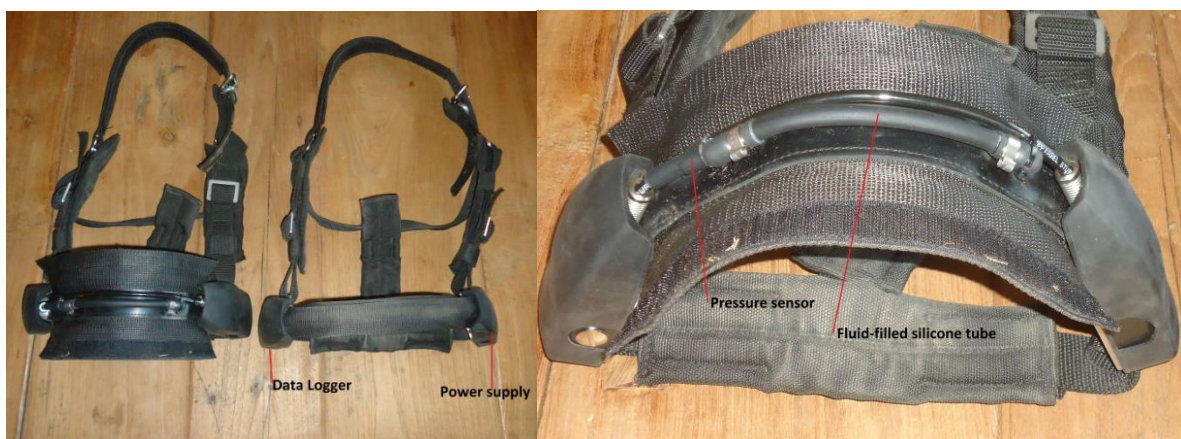
Figure 4: The build-up of an EquiWatchHalter with integrated sensor technology.
