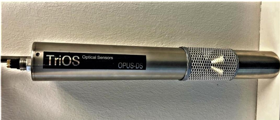
Figure 3. The spectral sensor OPUS deep sea with a self-constructed optical path protector grid.
