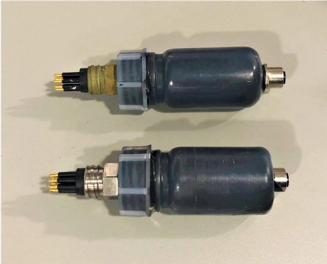
*Figure 2. Waterproof subcon-M8 adapters constructed for the tidal experiment.*
