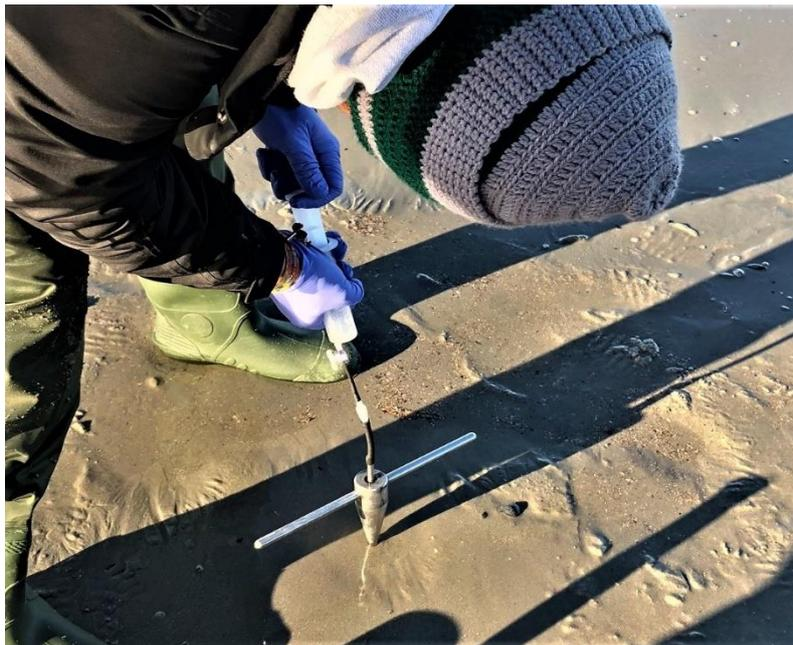
Figure 6. Collecting pore water samples along the onshore transects using a pore water lance.
