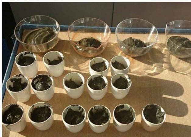
Figure 13 Samples right after sectioning filled in quartz and fireclay crucibles (Photo: Sylvia Schuster).
