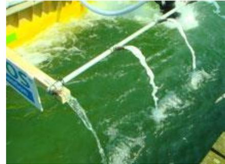
Figure 30 Spraying system used for Phoslock® applications. The spray bar can be hung in the hypolimnion or above the surface (Phoslock, 2015).
