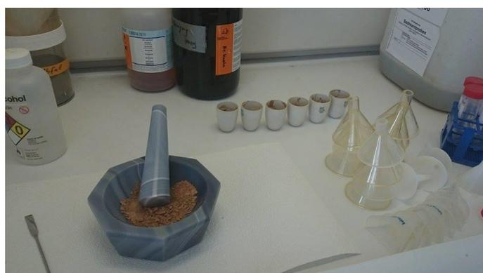
Figure 14 Mortar used for grinding of the samples (samples are in the fire clay crucibles) (Photo: Sylvia Schuster).
