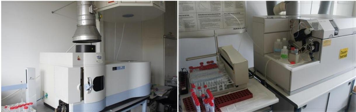
Figure 16 Inductively coupled plasma mass spectrometry device ICP-MS 7500c by Agilent Technologies and Inductively coupled plasma atomic emission spectroscopy ICP-OES by Perkin Elmer at the UFZ, Magdeburg, Germany (Photos: Sylvia Schuster).
