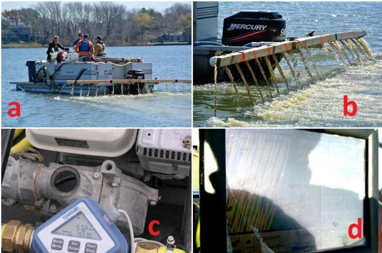
Figure 4 Swimming platform (a) with spraying system in detail (b) (27East.com). Picture of a flow meter (a) and a GPS system (d) used in the field by Dr. Yasseri (Photos: S.Yasseri, n.d.).
