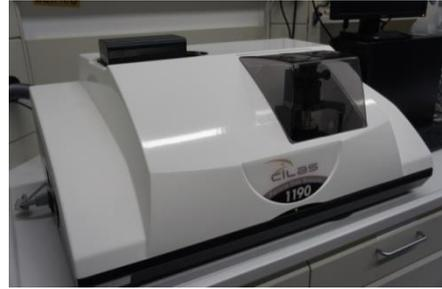
Figure 11 Cilas 1190 Particle-Size-Analyser used at UFZ, Magdeburg, Germany (Photo: Sylvia Schuster).
