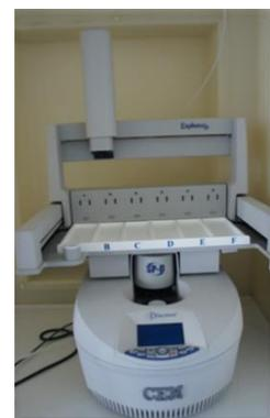
Figure 15 Microwave pressure digestion device by the company CEM (Photo: Sylvia Schuster)
