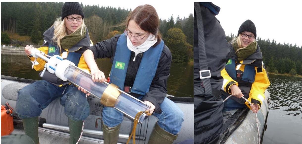
Figure 6 Preparing the MONDSEE CORER to lower it to the lakebed. The corer is secured with a rope (Photos: Martin Schultze).
