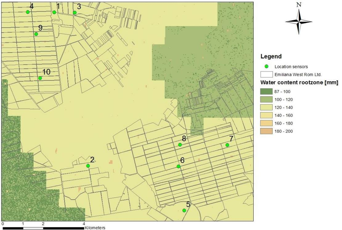
**Figure 4-7: Water content root zone - DACOM vs. Model, 28<sup>th</sup> June 2013**
