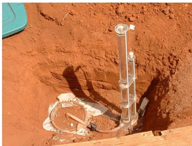
Figure 32: Tensio infiltrometer<sup>26</sup>.
