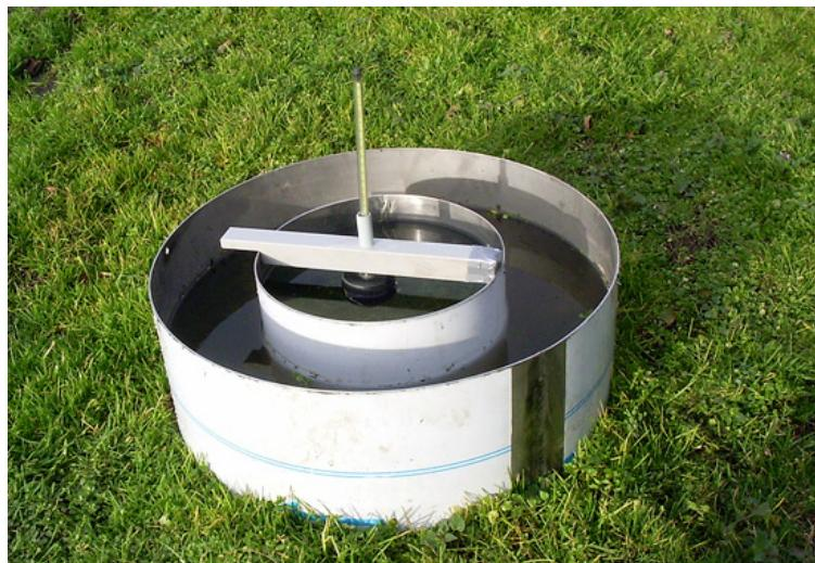
Figure 34: Double ring infiltrometer<sup>27</sup>.
