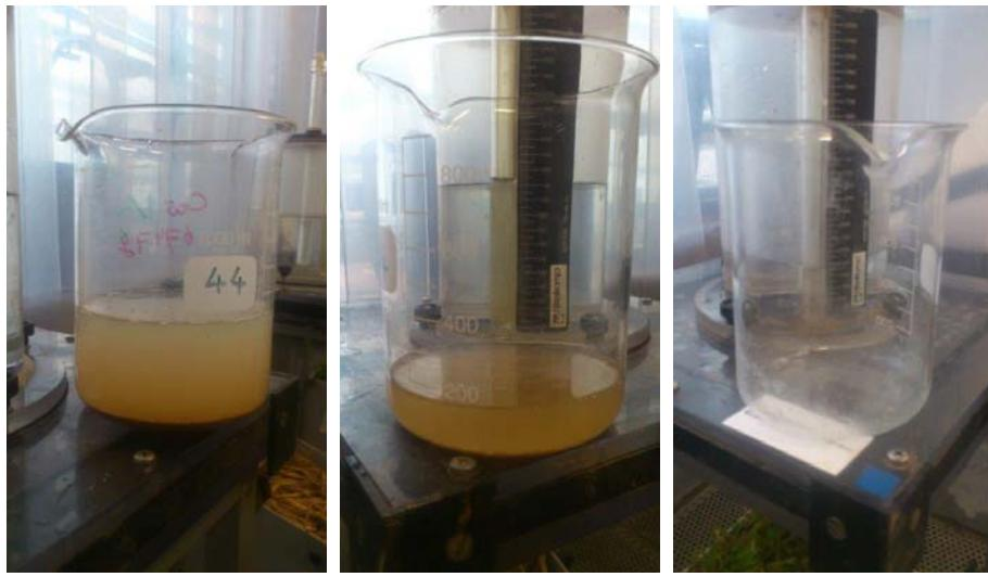
Figure 39: run off samples from left to right: bare soil, straw cover and grass cover.
