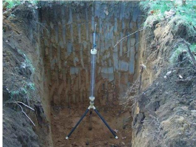
Figure 40: Guelph infiltrometer<sup>29</sup>.
