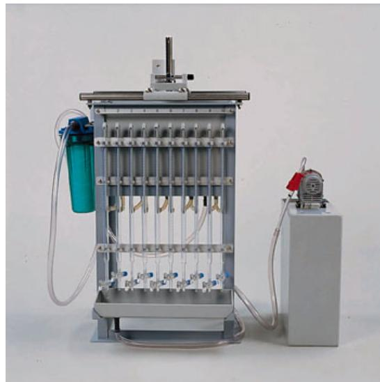
Figure 43: Labtype permeameter<sup>32</sup>.
