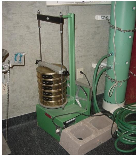
Figure 48: Grain size analysis<sup>33</sup>.
