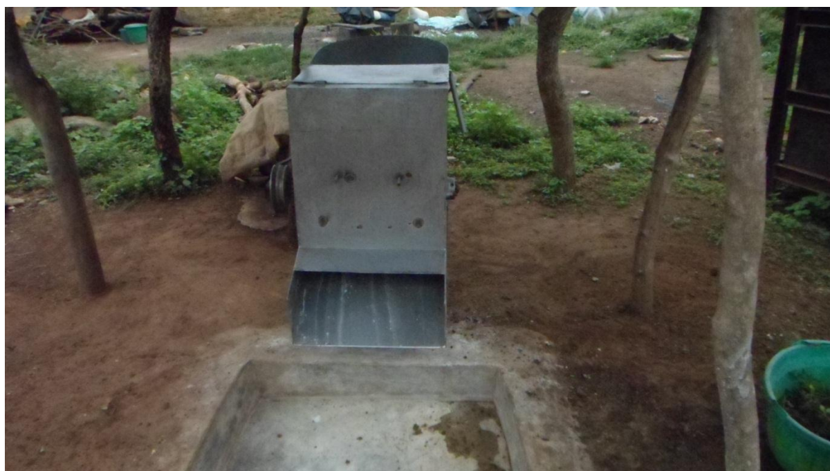
Figure 5.4: Steel Cassava grater donated by C:AVA to Gari Processing group
