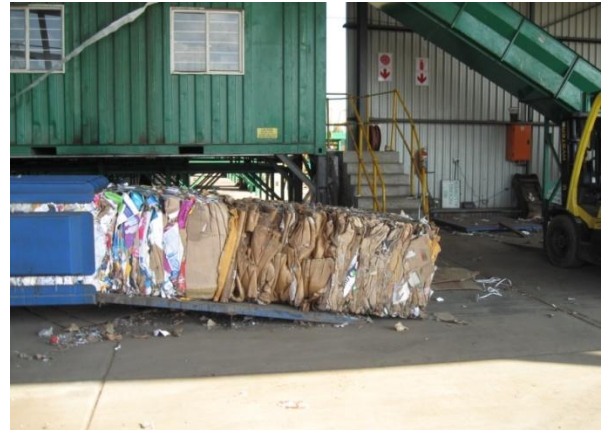
Picture 12: bails from the bailing machine
