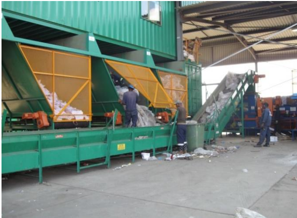
Picture 9: Empty waste bin after separation. The waste goes on the conveyor belt. the conveyor belt goes to the bailing machine
