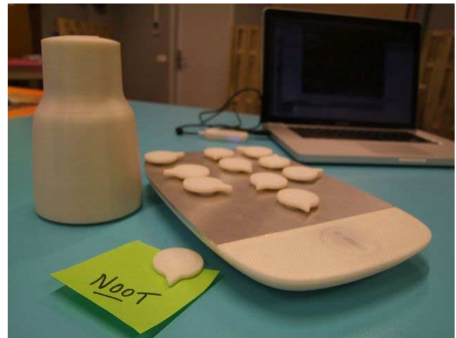
Figure 8. The final NOOT prototype. From left to right: audio-playback, a clip on a sticky-note, the dispenser tray and the central computer. Physical design by Van Berlo
