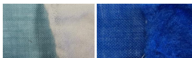
Figure 15 Colour Change: before and after washing test (Naturally dyed vs. Reactive dyed sample)
