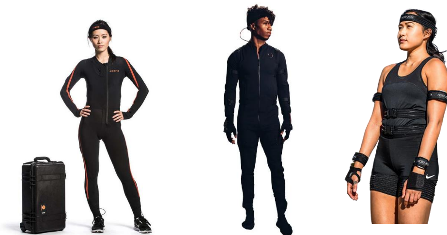
Figure 6 Three different inertial full body motion capture systems. From left to right: Movella's (Xsens) Link suit, Rokoko's Smartsuit Pro II and Noraxon's Ultium Motion Straps with trackers.
