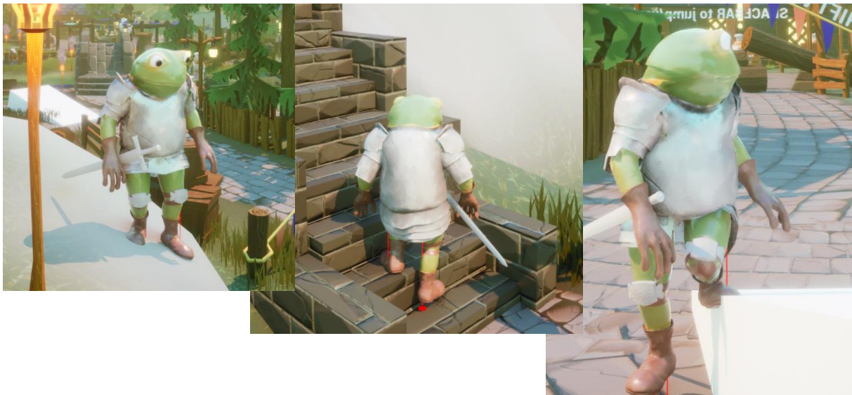
Figure 18 Test images for the IK foot placement tool, testing on slopes and steps in the game, altering the default idle animation provided by MVN recordings. Note the red line traces detecting the surface level and forwarding that information to the IK goal of the feet.
