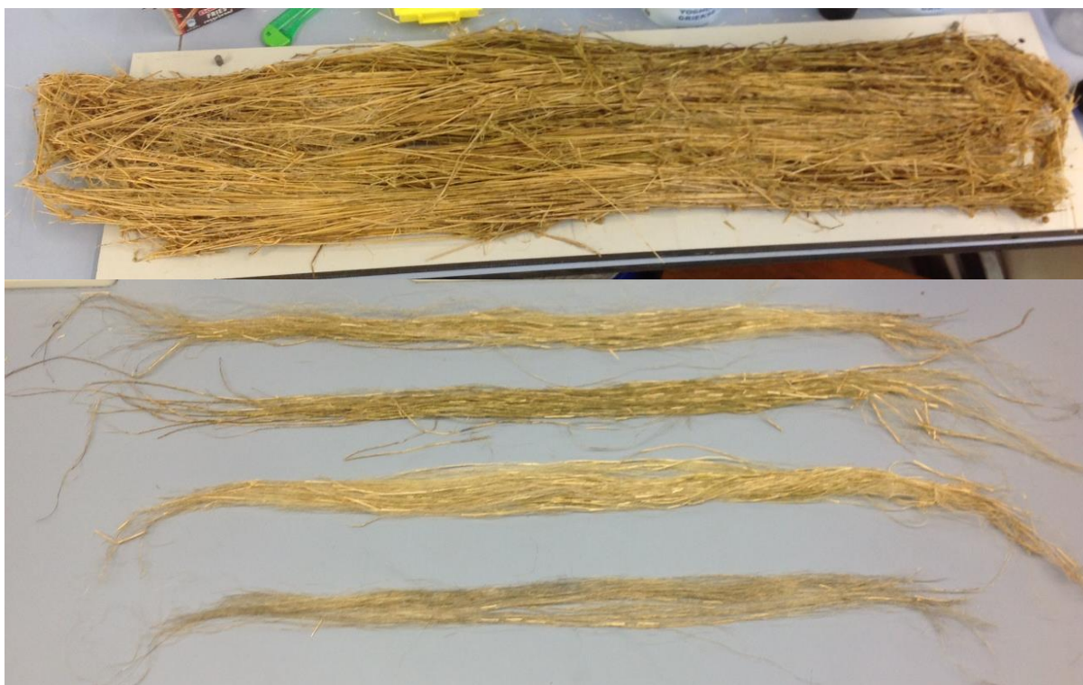
Figure 3-16: Long flax-fiber production with rotating drum and bubble column. (A) Flax bundle from rotating drum (B) Close-up of retted flax in a bundle (C) opened flax bundle (D) Long flax fiber production from bubble column.
