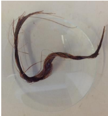
Figure 3-22: Flax fiber obtained during lab-scale retting processes with pyrolysis oil as conservator.
