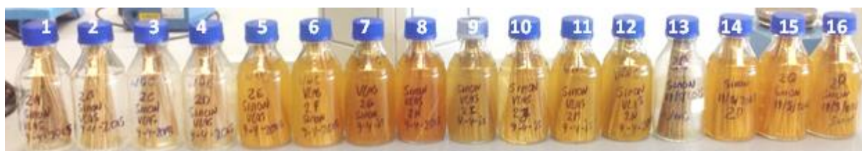
Figure 3-1, batch retting experiments. The bottles#1 and #2 are blanc. The bottles #3, #4 and #13 are dew-retting experiments. All other bottles contain water.
