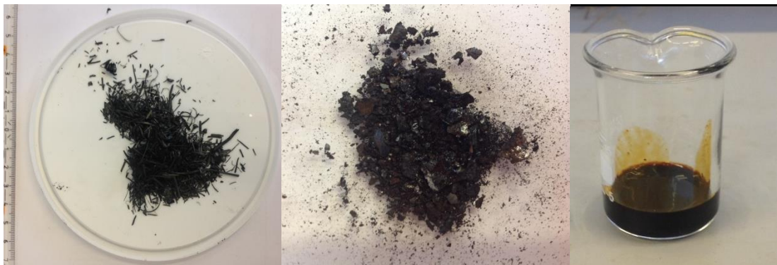
Figure 3-21: Photo of the pyrolysis products: 1. Charcoal 2. Probably carbon crystals 3. Pyrolysis-oil
