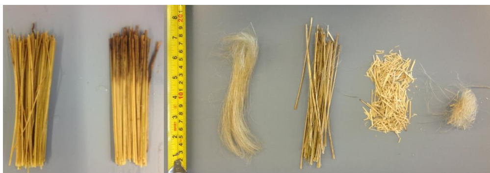
Figure 3-12B , Lab-scale experiments and processing after retting. From left to right: (1) Water-retted flax stems. (2) Flax stems that were partly water-retted and partly dew retted. The upper darker part is dew retted. (3) Short fibers. (4) Corresponding retted and dried stems. (5) corresponding shives. The shives are clean and regarding the size of the shives (2 cm long) it was separated easily from the fibers. (5) A cloud of short fibers that was obtained during the separation of the shives and the fibers.
