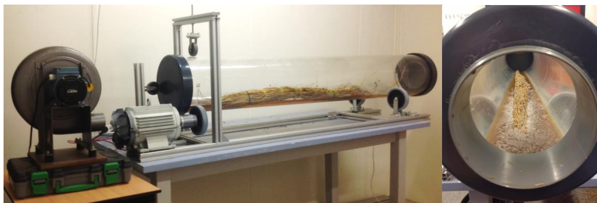
Figure 3-15: Set-up of the rotating drum for flax. The fan is needed to cool the motor. The motor is equipped with an internal cooling system, but this internal cooling system is only effective at a high rotation speed. Flax and water can be added via the side of the drum. During the retting process, the water takes up natural compounds from the flax stems (on the right).
