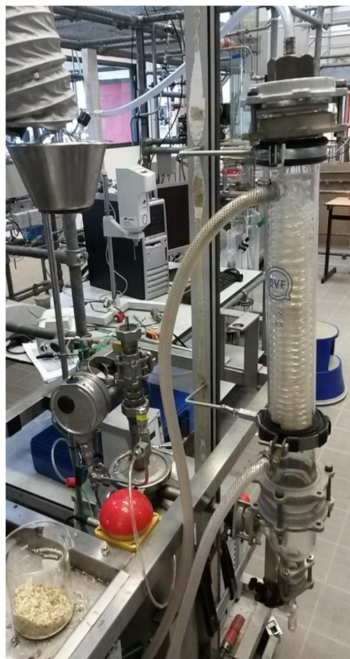
Figure 3-19, Schematic overview and photo of the pyrolysis system used. The pressure valve is to avoid overpressure of 0.5 bar in the reactor.
