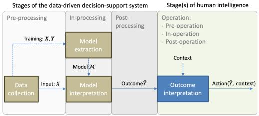
Figure 2: An illustration of the issue discovery and mitigation stages in an extended datadriven decision support system
