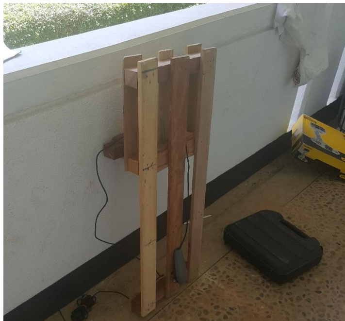
IMAGE 14: THE MODIFIED PALLET WITH THE FISHFINDER'S TRANSDUCER ATTACHED
