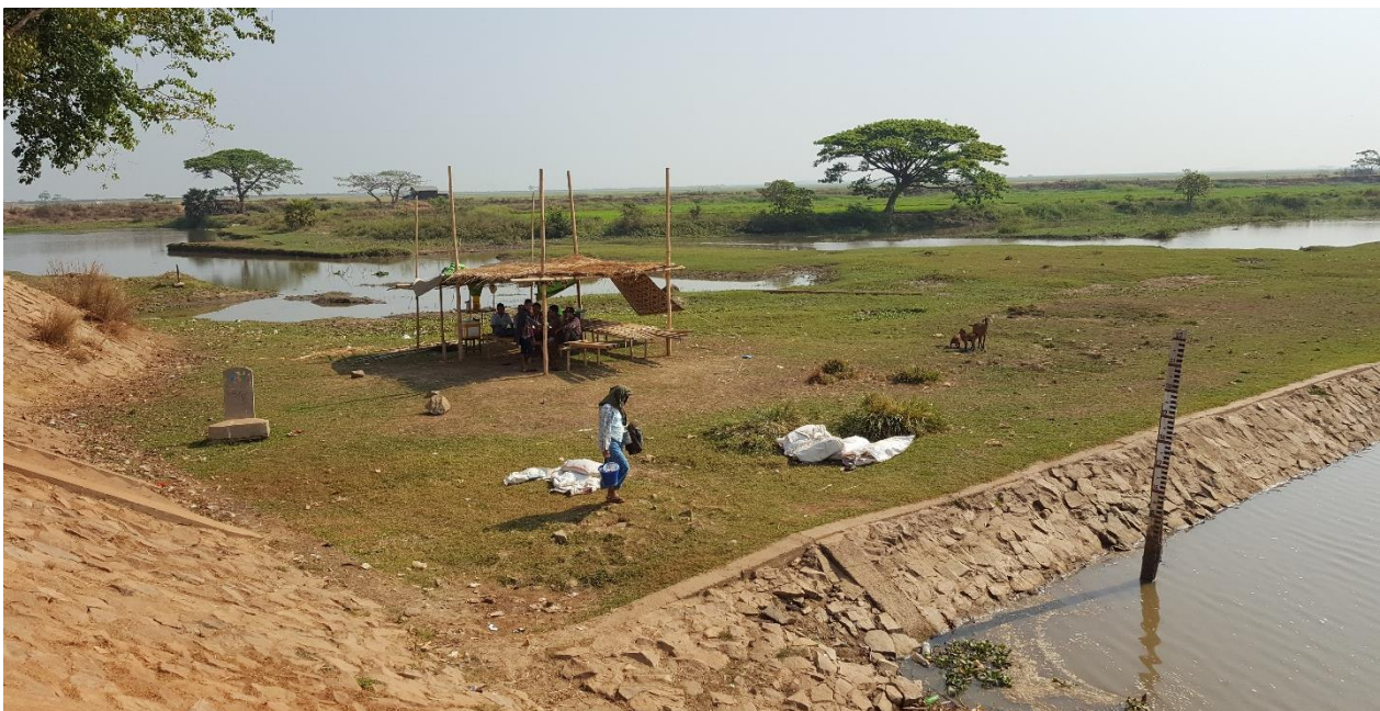
FIGURE 7: WATER LEVEL MEASURING AT THE DRAINAGE CANAL SIDE OF THE SLUICE GATE
