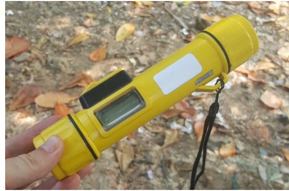
IMAGE 8: THE HONDEX PS-7 LCD DIGITAL SOUNDER
