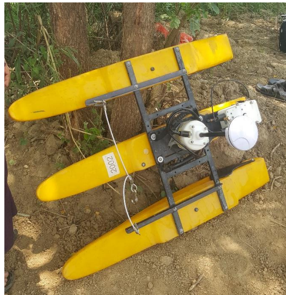
IMAGE 7: THE SONTEK M9 AND ITS FLOATING CONSTRUCTION
