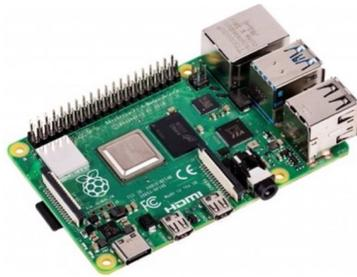
Figure 2.5: Raspberry Pi 4 model B [18].
