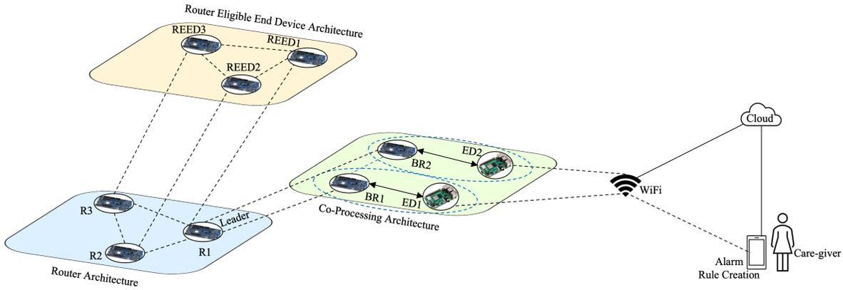
Figure 4.1: Thread network topology of the prototype.
