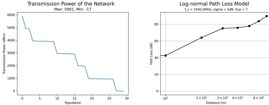
Figure 5.9: GA transmission power optimization based on different parameters. Figure 5.10: Path loss based on different parameters for large distance.
