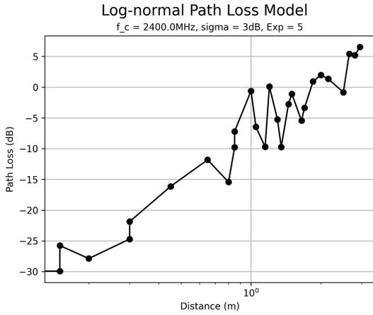
Figure 5.7: Path loss for lab location.
