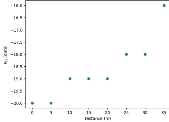
Figure 5.6: Transmission power vs. distance for home location using GA.
