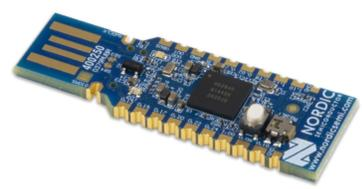
Figure 2.3: nRF52840 Dongle [16].
