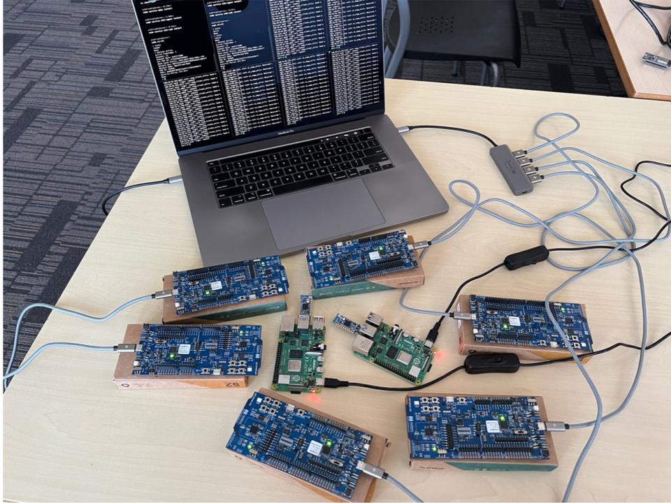
Figure 4.2: Thread network prototype setup in the lab.
