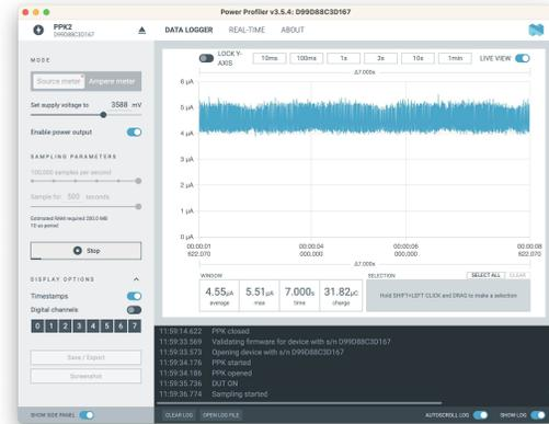
Figure 4.6: PPK II software in source meter mode.
