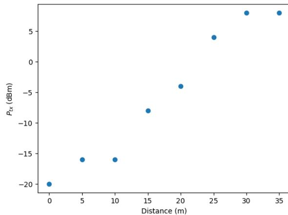
Figure 5.3: Transmission power vs. distance for lab location using MCM. Figure 5.4: Transmission power vs. distance for home location using MCM.
