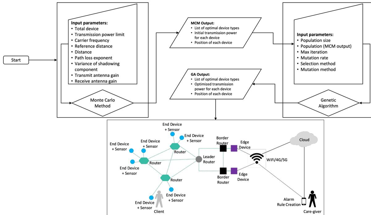
Figure 3.1: Thread network power optimization conceptual model.
