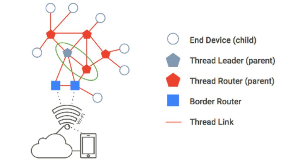
Figure 2.1: Basic Thread network topology [3].
