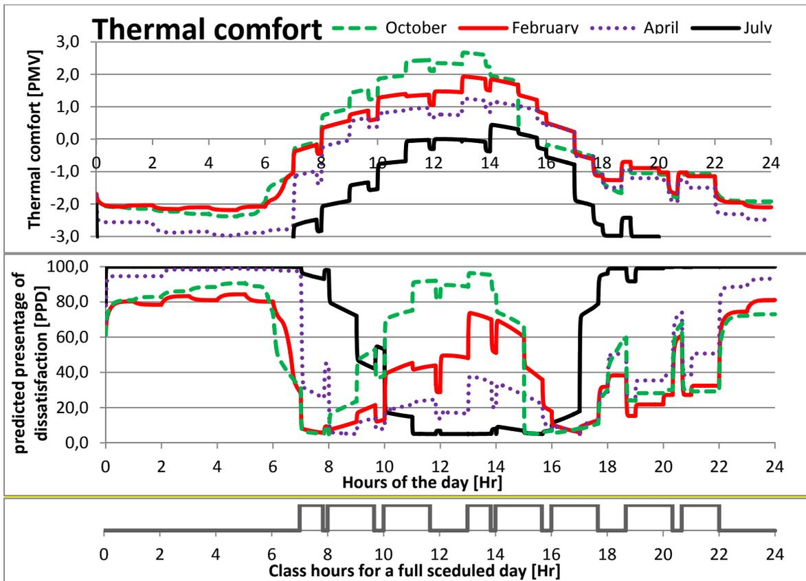
Figure 21: Thermal comfort in different seasons while using the solar chimney without air-conditioner. The lower graph predicted percentage of dissatisfaction as a function of only the PMV using Eq. 75.
