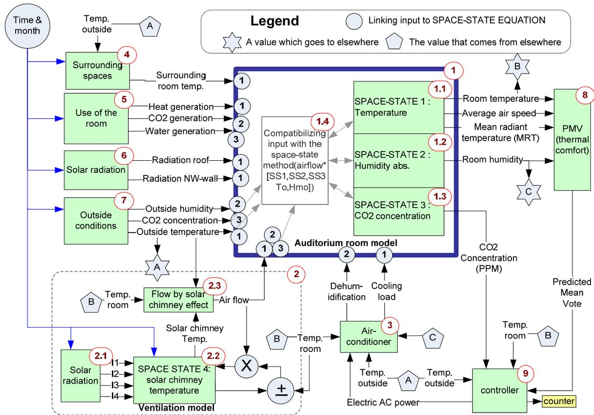
Figure 1: VISIO block scheme displaying the Matlab model
