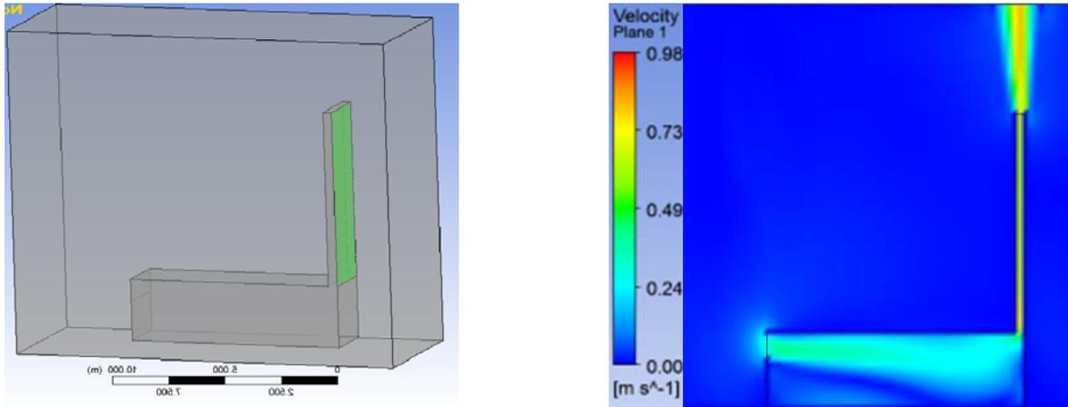
Figure 10: The model and the flow rate distribution which is established in the auditorium
