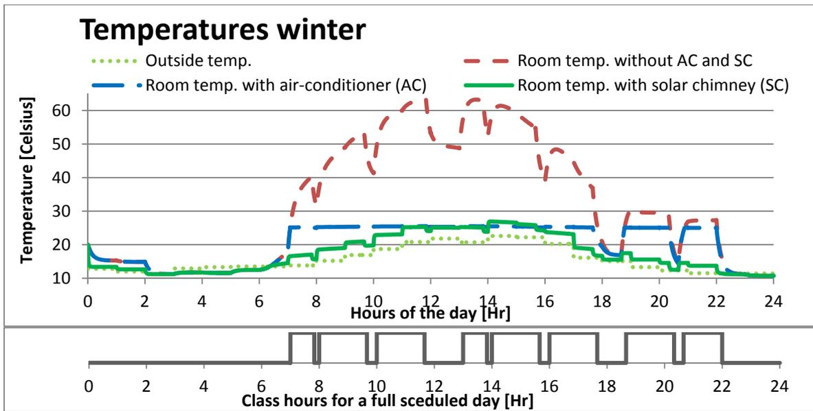
Figure 17: The room temperatures in the winter (15th of July ) for case 1, 2, 4 and the outside temperature.
