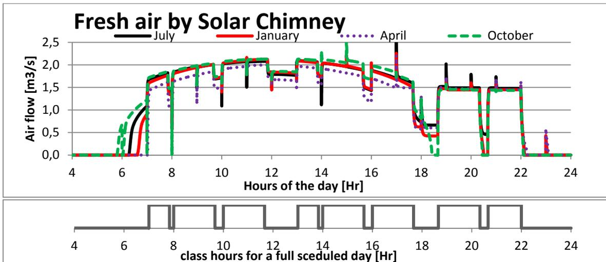
Figure 22: Air flow during the day for the four seasons caused by the solar chimney, while not using an air-conditioning.
