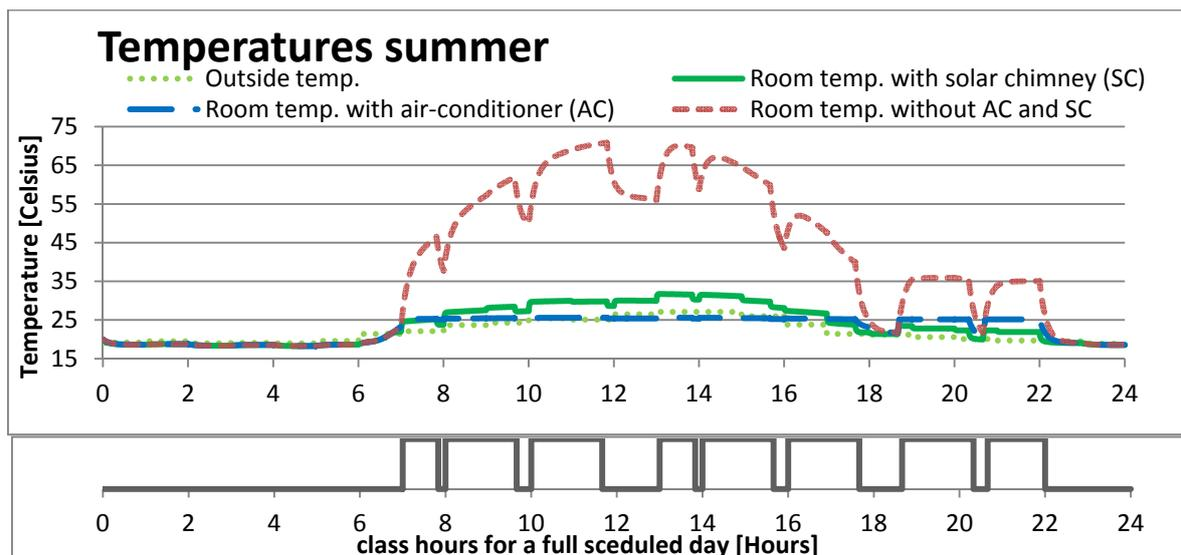
Figure 15: Above shows the room temperature in the summer (15th of January) for case 1, 2, 4 and the outside temperature.
