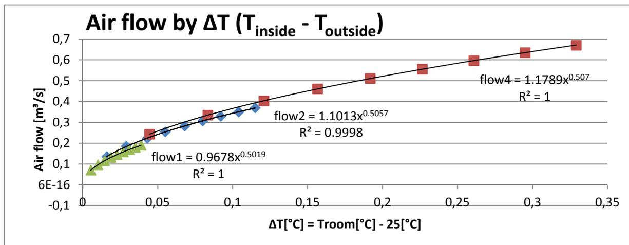
Figure 11: Correlations  $\Delta T(\text{outside temp} - \text{avg. inside temp})$  against air flow, for the configurations with a solar chimney of 1 meter high(flow1), 2 meter high(flow2) and 4 meter high(flow4).
