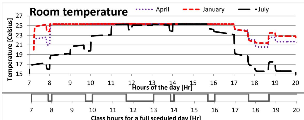
Figure 23: Thermal comfort for solar chimney integrated in an air-conditioned environment
