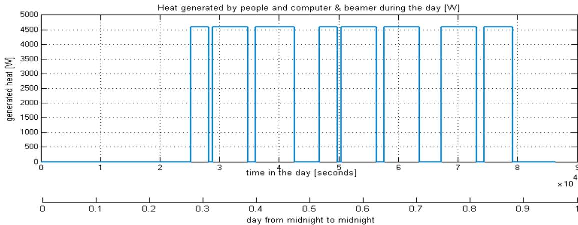
Figure 7: Heat added to the room by 30 people, lamps and one computer during the day
