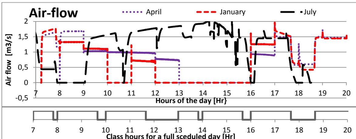
Figure 25: Air-flow generated by the solar chimney when the air-conditioner is active all day to keep the temperature below 25.3 degrees Celsius.
