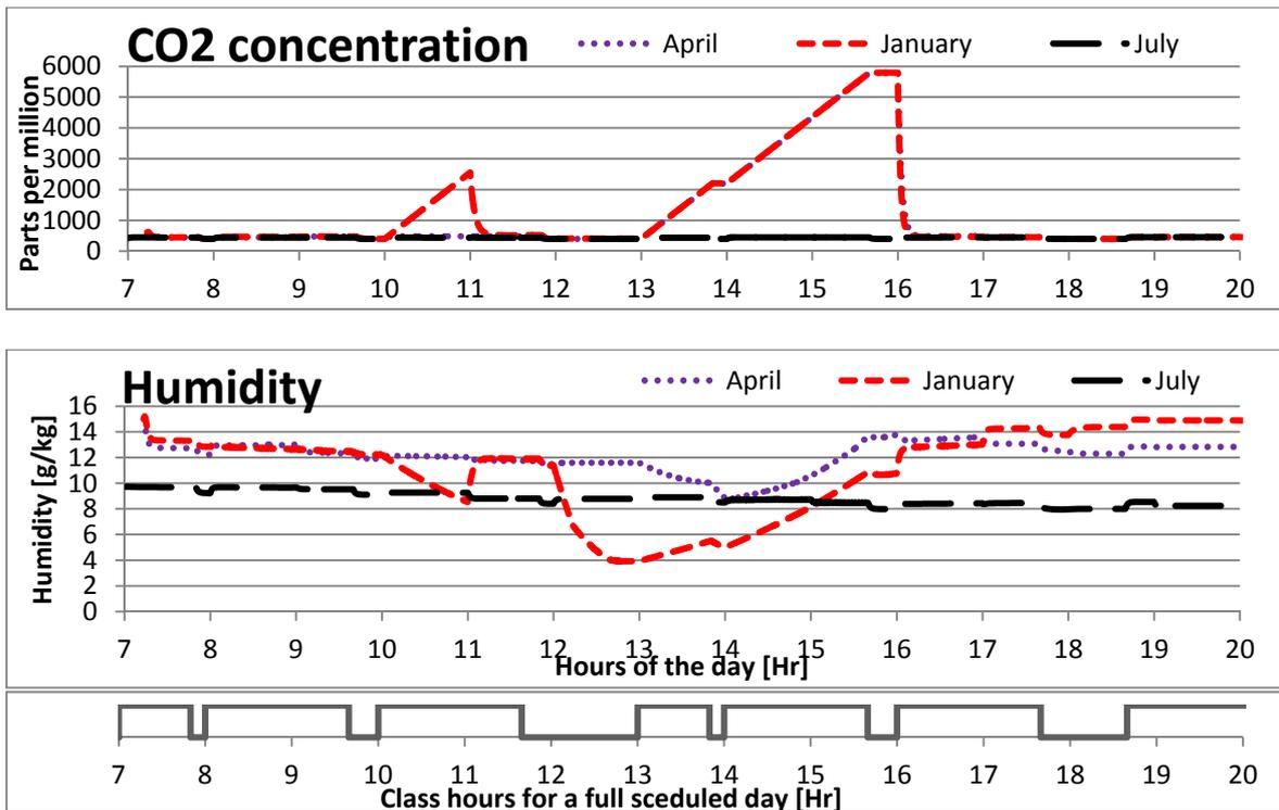
Figure 26: Air-flow and the air-quality measures CO<sub>2</sub> concentration and humidity for the course of a day in January, April and July
