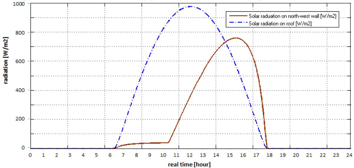
Figure 6: Radiation curves on the roof and wall of the auditorium for the 15th of July for midnight to midnight (without considering clouds)
