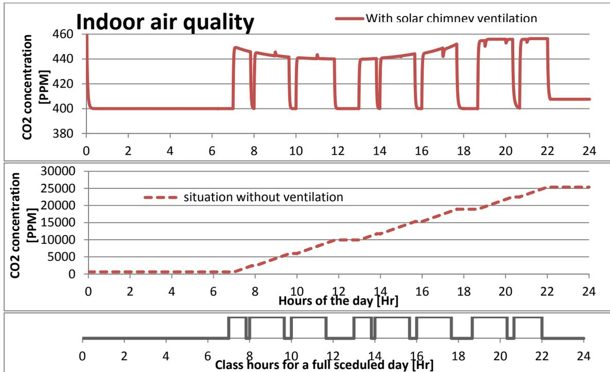
Figure 19: Above the CO<sub>2</sub> concentration when using the solar chimney (without AC) in February, promoting a high air quality. Below the CO<sub>2</sub> concentration without any ventilation, going up to unappreciated levels within one day
