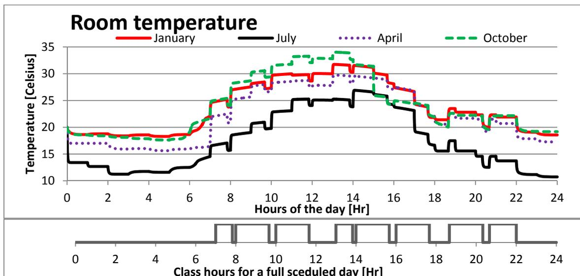
Figure 20: Room temperature using the solar chimney and without using the air-conditioner.
