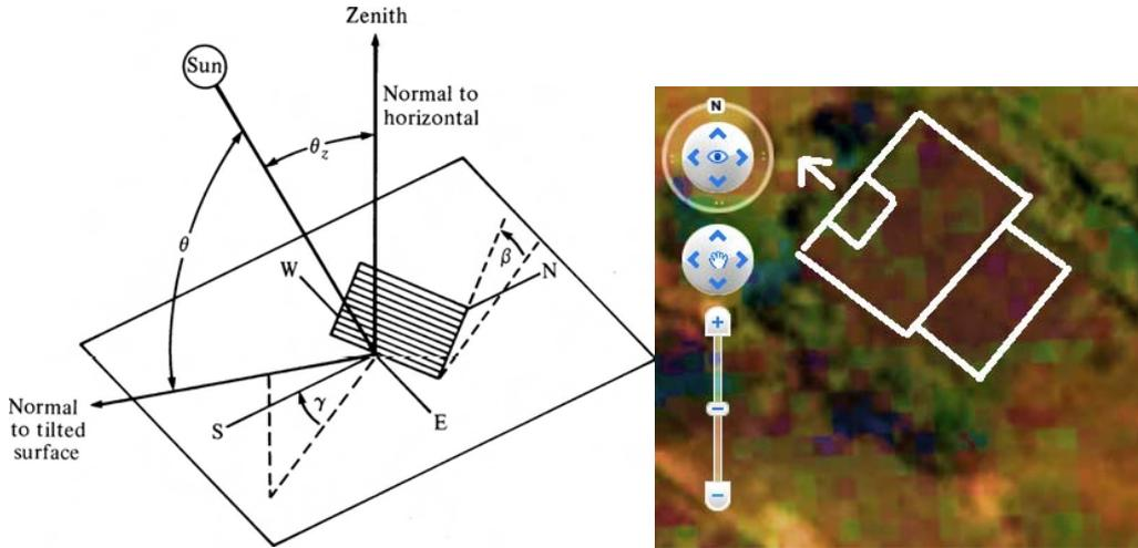
Figure 5: Zenith angle  $\theta_z$ , angle of incidence  $\theta$ , slope  $\beta$  and azimuth angle  $\gamma$  for a tilted surface. (Note: for this easterly facing surface  $\gamma < 0$ .) After Duffie and Beckman 1991.
