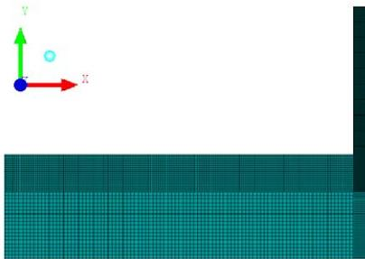
Figure 9: Mesh hexane dominant "type D", with elements of mesh size 0.1 m, 0.05 m and 0.025 m.
