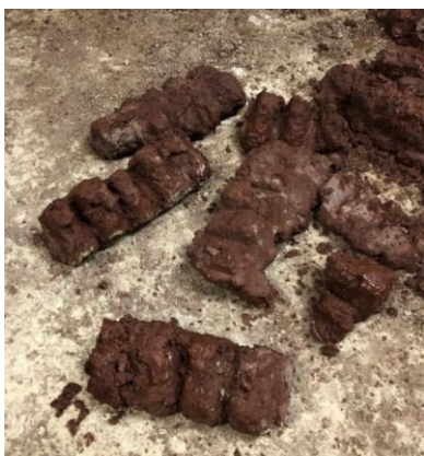
Picture 4.2 Material built-up in the mixer with higher percentage of \text{CaCO}_3 during plant-scale acidulation test.
