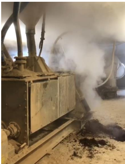
Picture 4.5 Steam formation due to water addition in SSP production
