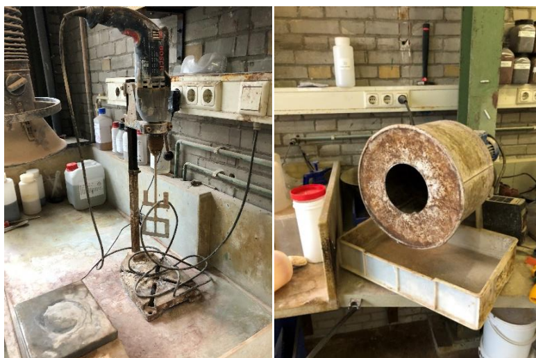
Picture 3.1 Pilot scale equipment: (1) the mixer and (2) granulation drum.
