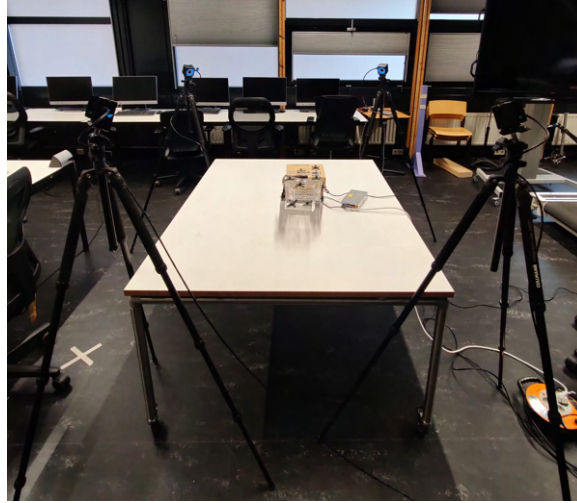
Figure 8: Camera set up - unloaded testing condition
