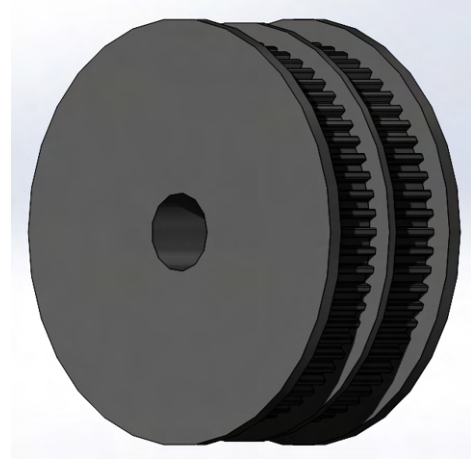
Figure 4: Adjustment radial-ulnar deviation gear, part of figure 2F
