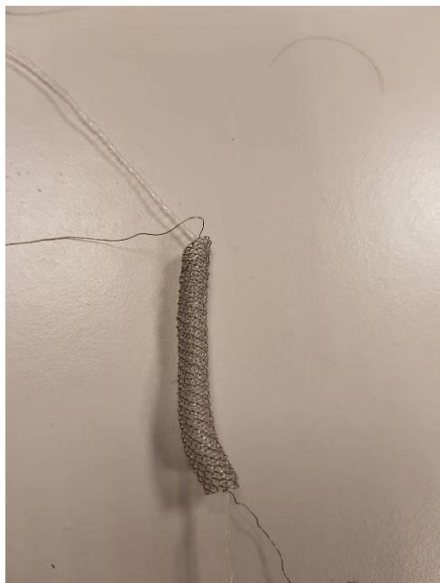
Figure 1.13 Completed artificial muscle, note: not the same one as in figure 1.12. This one can be seen in chapter 6.
