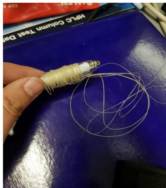
Figure 4.7: First successful batch of extruded PA6, 0.6 mm with a larger variance than the ABS extruded in figure 4.6.
