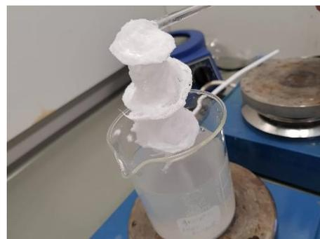
Figure 5.1 PA6 precipitate after formic acid dissolving.
