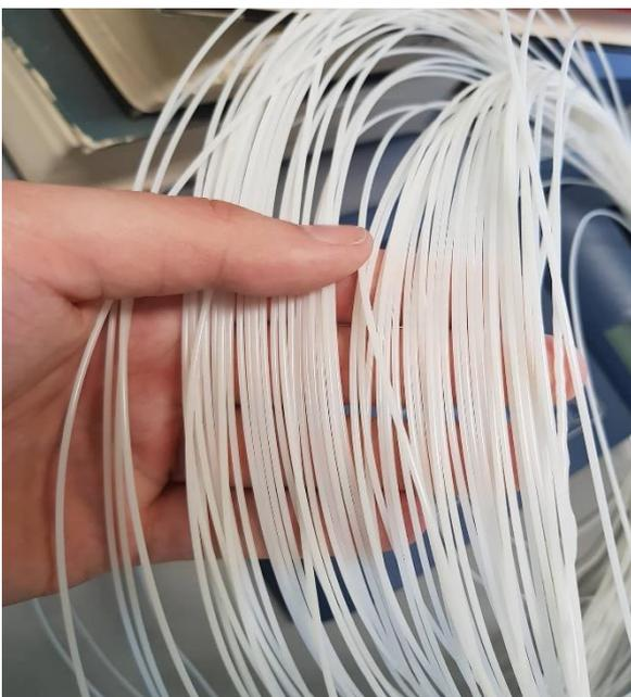
Figure 4.6: First batch of ABS extruded using the filastruder. As can be seen the overall diameter variance is fairly low.
