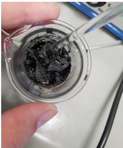
Figure 5.3: Nylon 6 (90%), graphene (9%), and graphene-oxide (1%) polymer composite produced through melt compounding.
