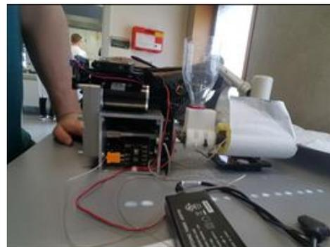
Figure 4.2: Mechanical assembly of the filastruder completed, part 2/2.
