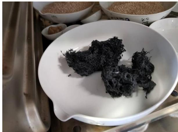
Figure 5.2: nylon 6 (90%), graphene (9%) and graphene-oxide (1%) polymer composite produced through the formic acid dissolving production method.
