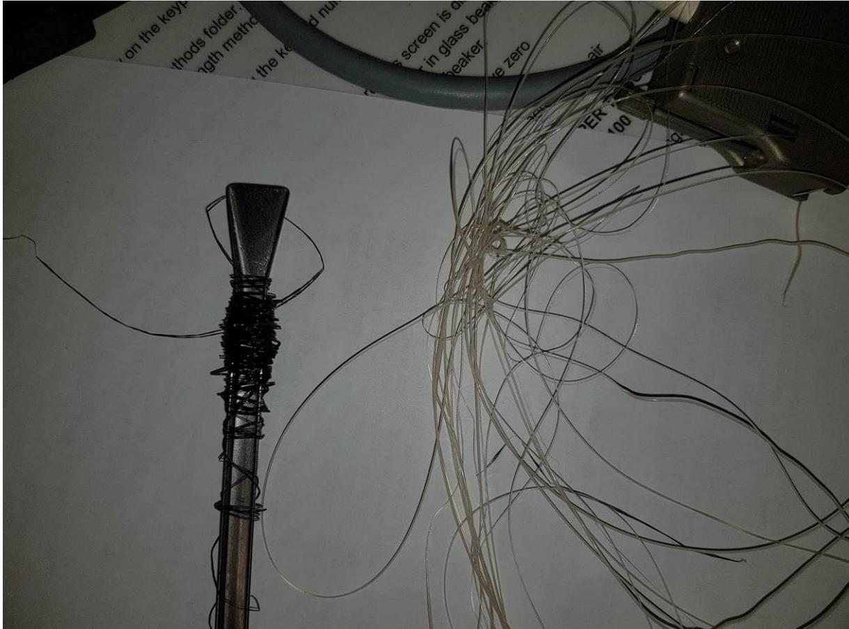
*Figure 6.6: 9% Graphene, 1% graphene-oxide, 90% nylon composite wire on the left, compared to regular nylon 6 wire on the right. It is clear that the wire on the left is black while the regular nylon is a light yellow/white colour.*
