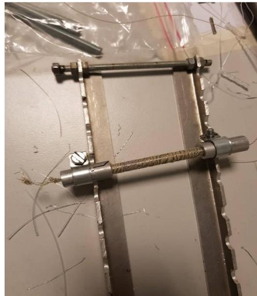
Figure 1.12: example of an artificial muscle, the quality of which is poor, however this is first trial with extruded nylon 6.
