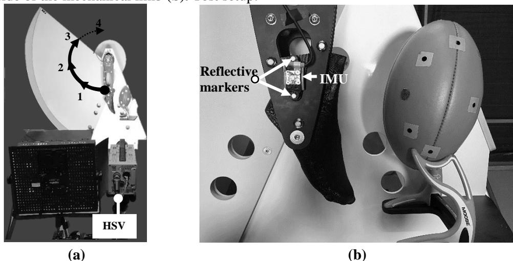
A high-speed video (HSV) camera (Photron SA3, Photron Inc., USA) data logging at 1000 Hz was used to identify ball contact (BC), ball release (BR) and calculate foot velocity of the mechanical
