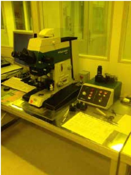
Figure 17: Photo of Bright field optical microscope
