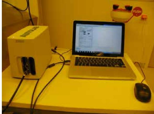
Figure 10: Photos of experimental electroplating setup. On the left the electrochemical cell with the wafer. On the right the PGSTAT204 connected to a laptop running NOVA
