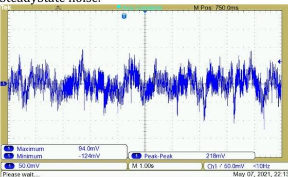
**Fig. 11** – AC measurement of the SteadyState performance during active feedback loop. Common deviation of 50 mV with occasional peaks up to 100mV.
