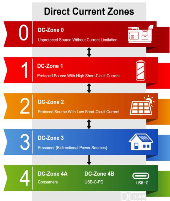
**Fig. 14** – DC-zones stated by the NPR9090[22]. Each zone is defined with criteria to connect the devices.
