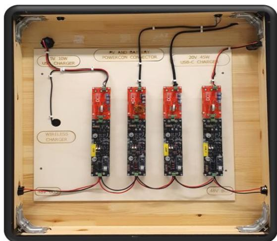
**Fig. 15** – Bottom-view demonstrative setup. All devices powered by U1L circuits are mounted underneath the table.
