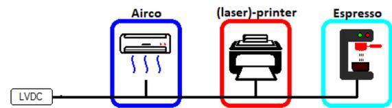
Fig. 4 – CASPOC Simulation model of an LVDC branch with three common components as active loads.
