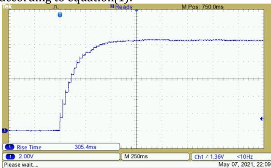
**Fig. 10** – Rise-time and Feedback-cycle time to reach 10 V SteadyState output.
