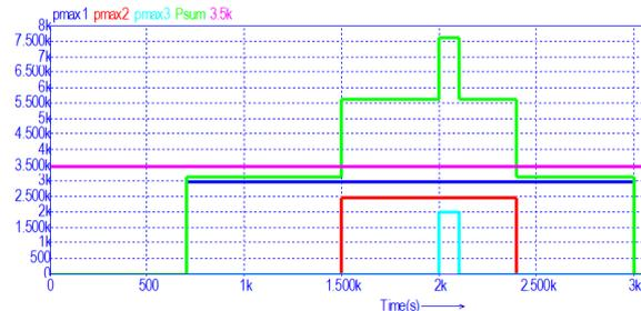
**Fig. 5** - AC system, the maximum power (pink) is exceeded as the total power (Green) increases. Fuse breaks.
