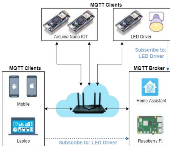
Fig. 2 – MQTT overview of the IoT DC-powered desk.
