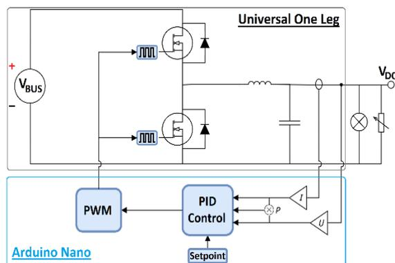
Fig. 3 – Schematic interaction U1L and Arduino Nano.
