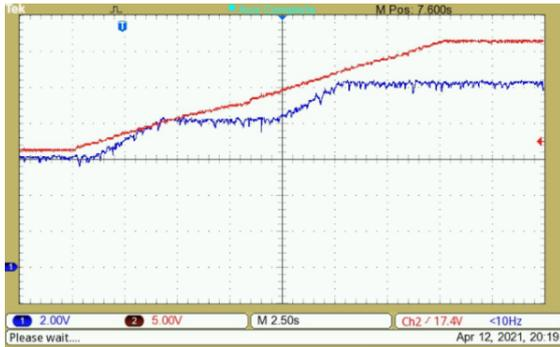
**Fig. 9** – A droop curve measured with an oscilloscope. As  $V_{bus}$  (red) changes, Voltage out (blue) dynamically changes along.
