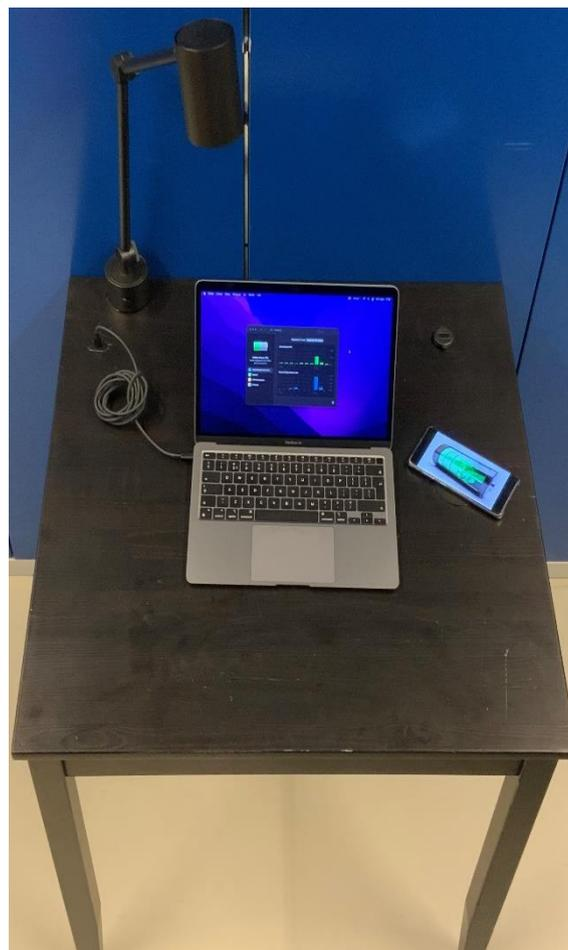
**Fig. 16** – DC-powered table placed in the living lab in the auditorium of THUAS, fed by a 48V battery. While charging the laptop and Phone with LEDs [23]
