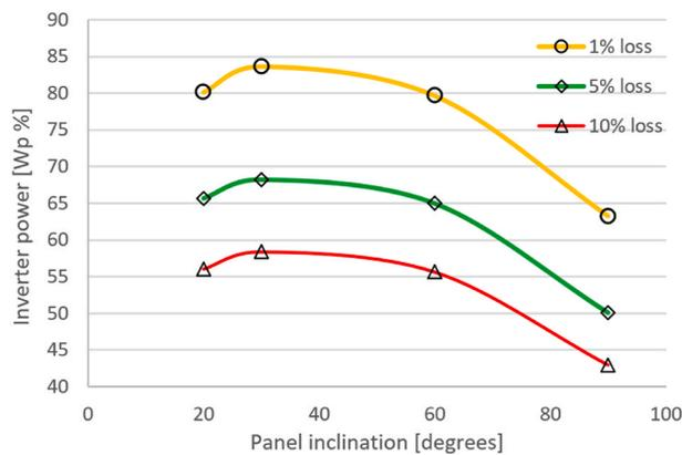
Fig. 14. Inverter power in % of the solar PV Wp as a function of slope of the solar PV panel for various energy yield losses caused by clipping of the inverter.
