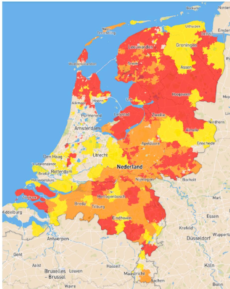
**Fig. 1.** Locations with a too weak grid provided by (Netbeheer-Nederland, 2021). With: a grid that does not allow the feed-in of solar and wind parks (Red), a weak grid with a preliminary notice on structural grid capacity problems (Orange), a grid with upcoming grid capacity problems (Yellow). (For interpretation of the references to colour in this figure legend, the reader is referred to the Web version of this article.)
