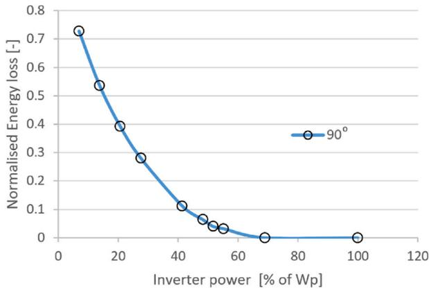
Fig. 13. Normalised energy loss of a facade panel (90°) as a function of inverter size (as a percentage of solar PV Wp, without inverter losses).
