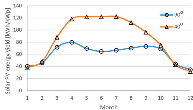
Fig. 12. Monthly energy yield of a facade panel ( $90^\circ$ ) of 1kWp for a South facing facade compared to the orientation for maximum energy yield, i.e. facing South at a slope of approximately  $40^\circ$ , according to (PVGIS, 2019).
