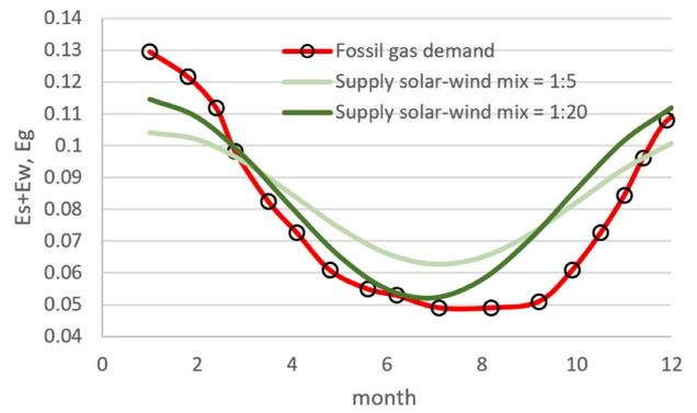
**Fig. 10.** Demand of fossil gas  $E_g$  based on the normalised data found in Fig. 7, mix of solar PV and wind energy supply  $E_s + E_w$ , with a ratio of respectively  $E_s : E_w = 1 : 5$  and  $E_s : E_w = 1 : 20$
