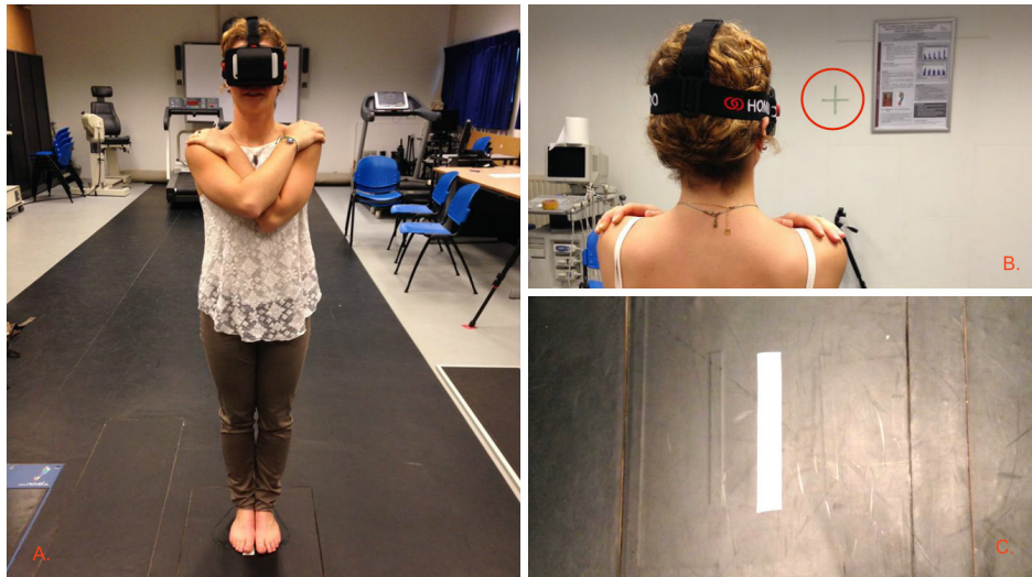
Figure 1: A. Positioning of the participants. Note: Medial malleoli touching together and arms are crossed to avoid compensations of the upper body. B. Forward direction marked with a cross (see red circle). C. The middle of the force plate was marked with a white line. Participants were asked to keep the line between their feet.
