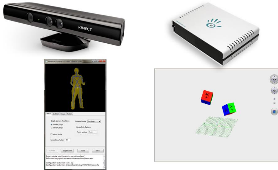
Figure 14 Microsoft Kinect and the PST live motion tracking
