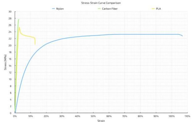
Fig. 2. Comparison of stress-strain graphs of some commonly used materials
