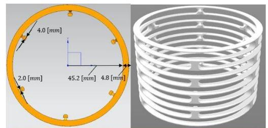
Fig. 10. RVS concept with supports for Sorbothane
