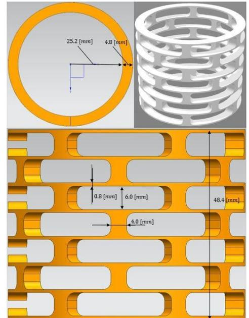
Fig 7: Nylon spring design
