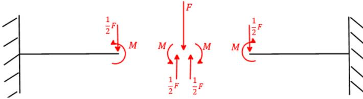
Fig. 5. Free body diagram beam
