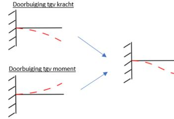
Fig. 6. Reaction caused by the force and moment
