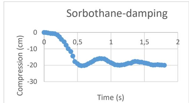
Fig. 9. Sorbothane compression over time
