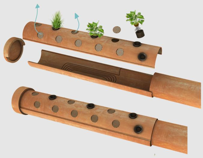
Passive Ventilation vents (windcatchers) lead hot and dry air into terracotta pipes, the end part is equipped with a patterned inner surface for maximum evaporation, the surface is saturated with water from roof what stormwater tank, to evaporating into the rooms cooling the air and humidifying it at once
