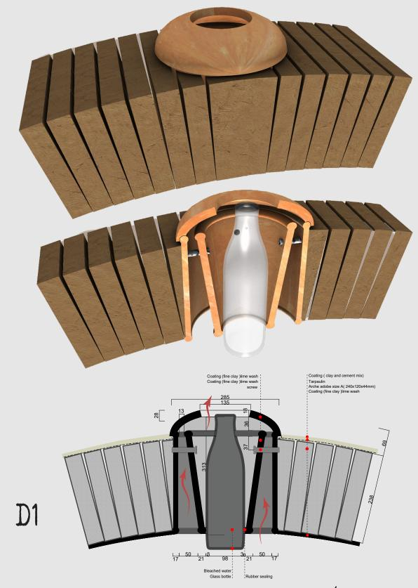
This low c solution for skylight (solar tube) is a placeholder for high-end one, the bleached water prevent modeling and scatter light more consistently, also this forms a protected outlet for hot air through the roof
