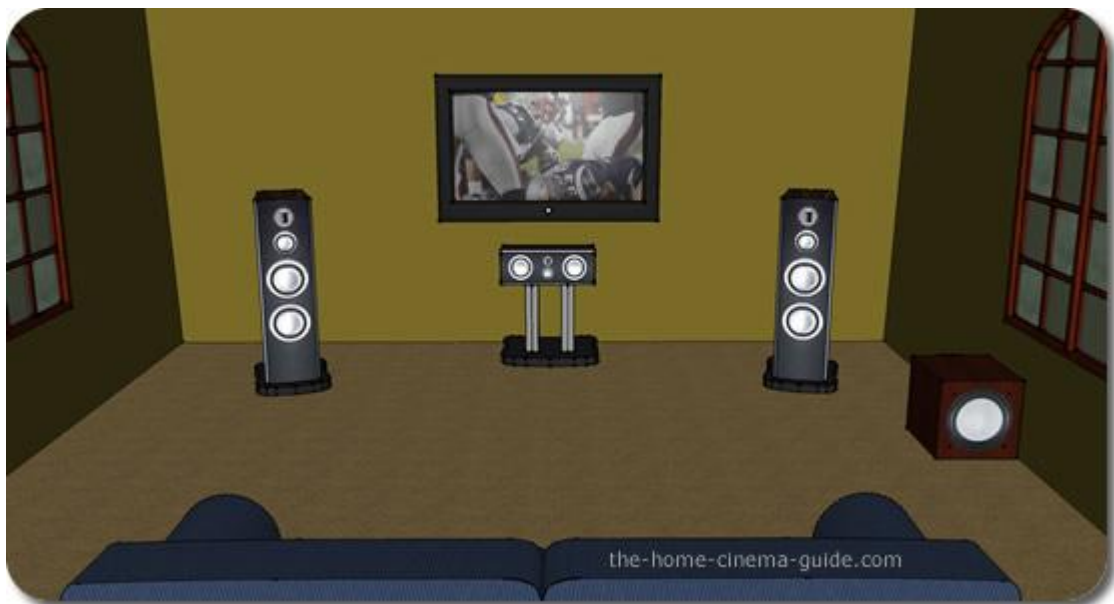
Figure 20. Recommended Front Speaker Placement
