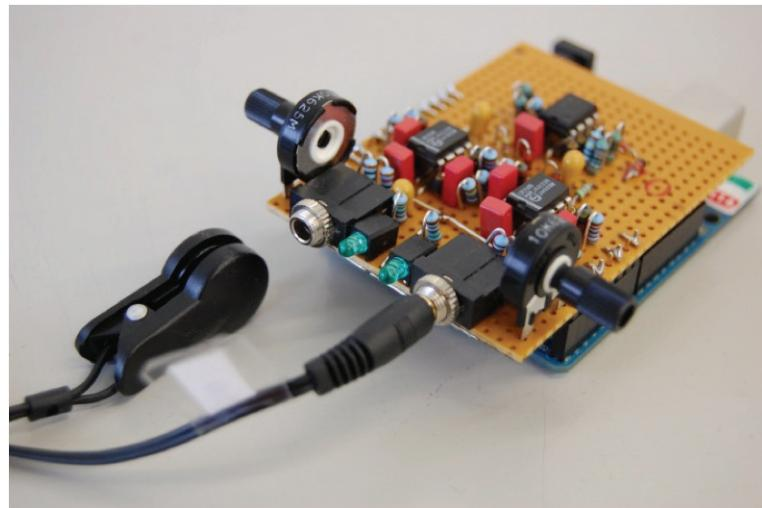
*Fig. 2.* A prototype for monitoring heart rate by means of the optical method of Photoplethysmography
