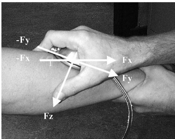
Fig. 1. Hand/palm held built-in 3D force sensor with local coordinate system.  $F_z$  represents the perpendicular force;  $F_x$  and  $F_y$  represent the shear forces.
