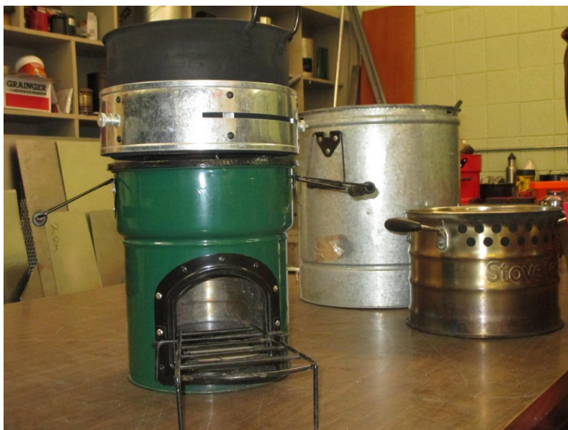
Several different kinds of rocket stove prototypes in the Aprovecho lab. (Jacob Lebel)
