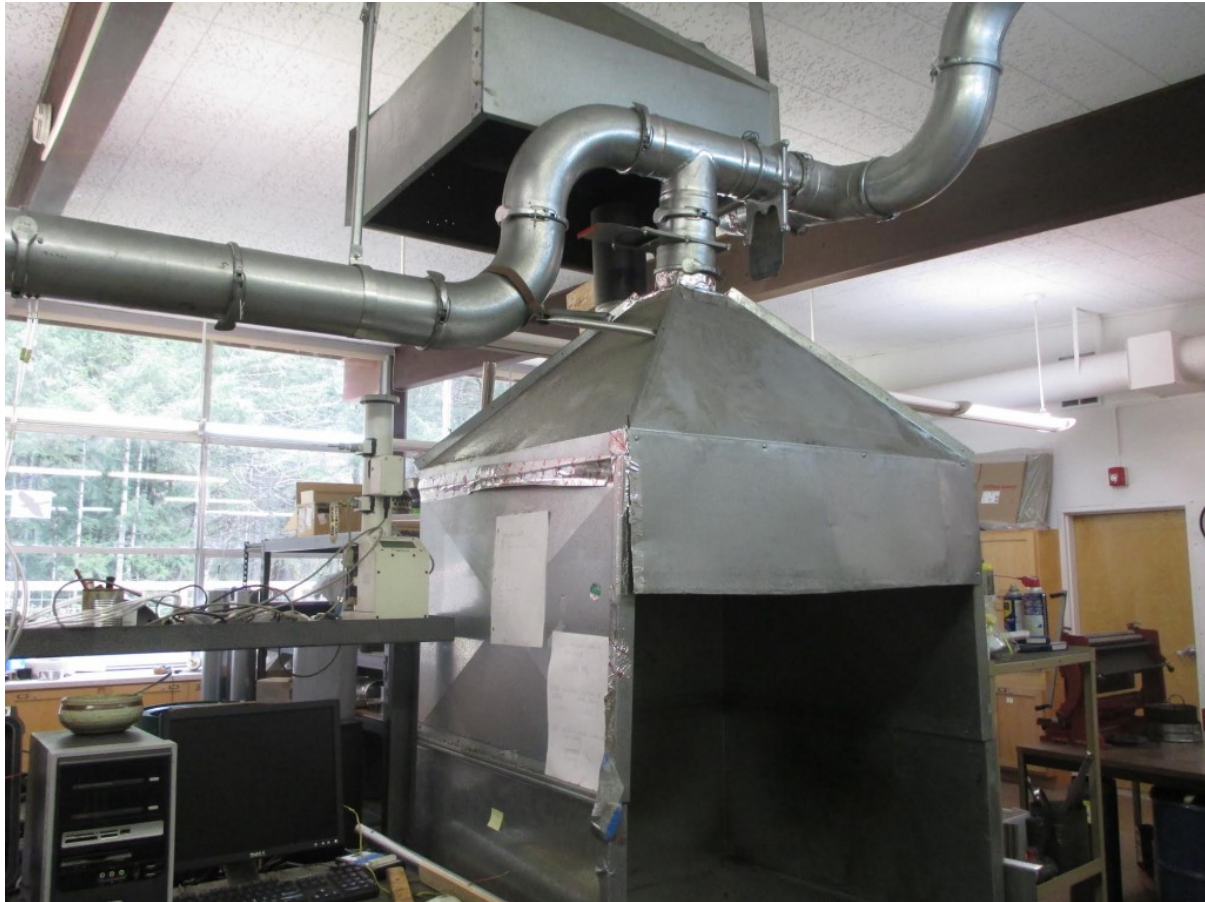
Laboratory Emissions Monitoring System developed by Aprovecho Research Center uses hoods with sensors connected to a computer to measure different molecular and particulate emissions. (Jacob Lebel)
