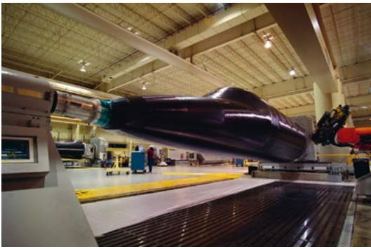
This business aeroplane is constructed fully automatically by applying carbon tape impregnated with synthetic resin layer by layer.
