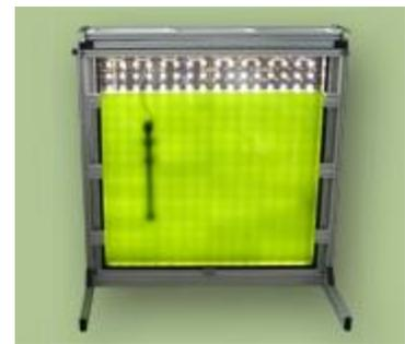
Figure 7-1 A small flat photobioreactor used for cultivation of phytoplankton (picture retrieved from: <http://www.psi.cz/>)
