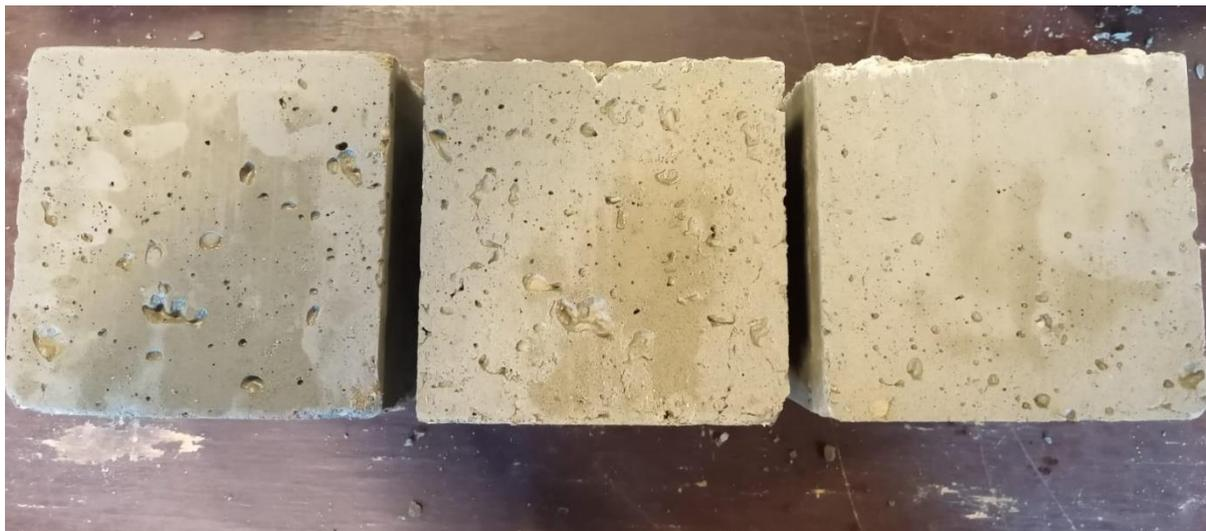
Figure 7: Ambient cured geopolymer concrete (Mix1) cubes in 7 days.
