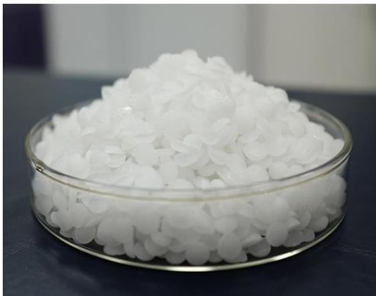
Figure 4: Sodium Hydroxide Pellets.
