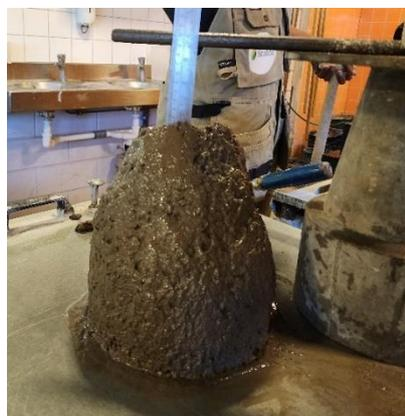
Figure 6: Slump reading of Mix 2.
