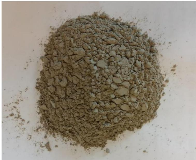
*Figure 2: Fly ash used in this study.*
