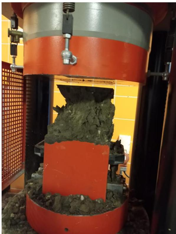
Figure 8: failed cube (Mix1) at 7 days
