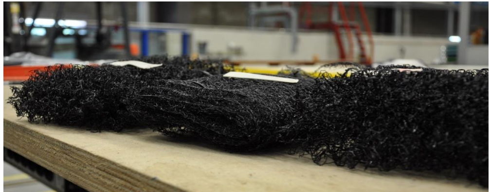
Figure 30: Three different type of permeable mattress materials
