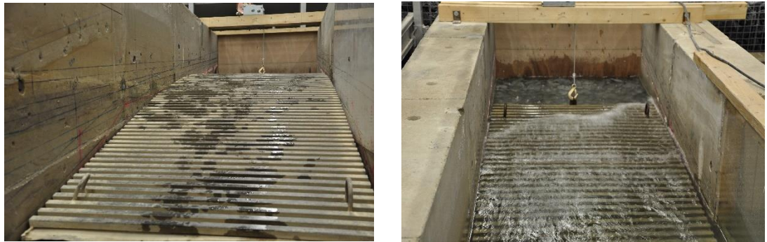
Figure 28: Physical design of the Parabolic damper slope used as model 2A and 2B.
