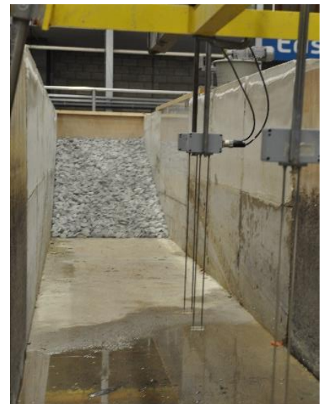
Figure 38: Flume inside the Pacific basin where the experiment models were installed.
