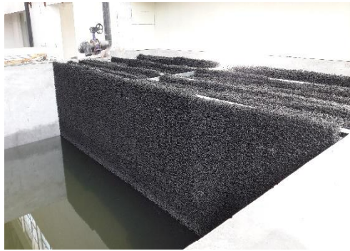
Figure 9: Mattress placed vertically at the end of the basin for wave absorption in China, Courtesy: Deltares
