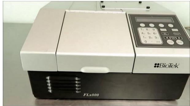
Figure 15 Biotech microtiter plate reader Fx800
