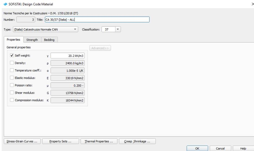
Figure 70: Design code material - Alternative 2
