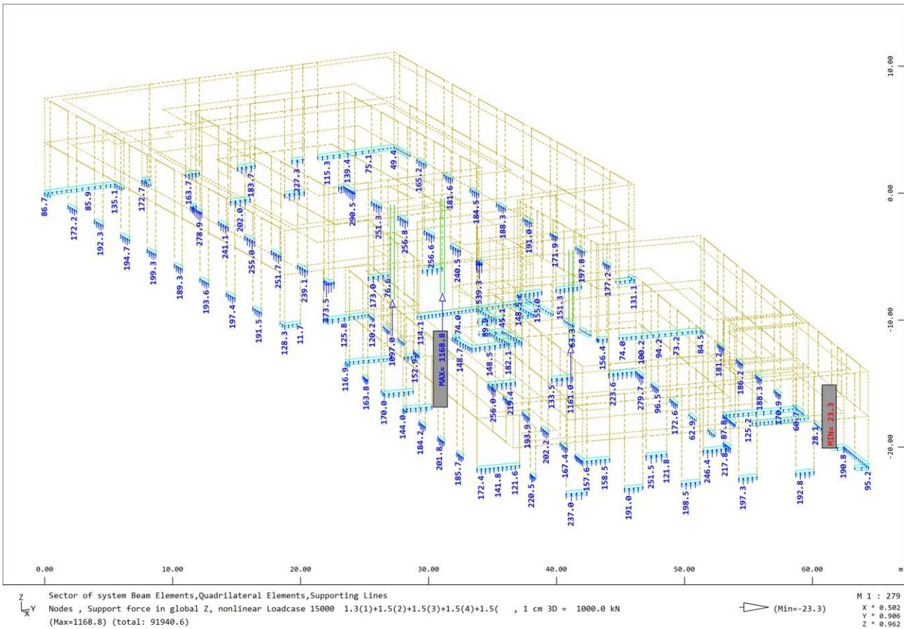
Figure 95: Support reactions - lightened model
