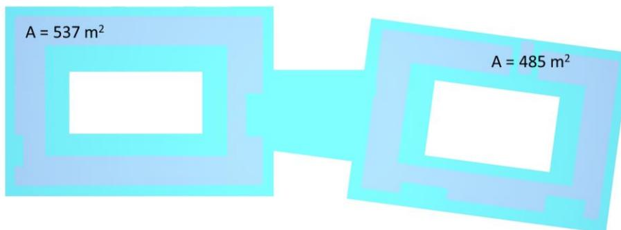
Figure 87: Relieved portions - First-Floor slab
