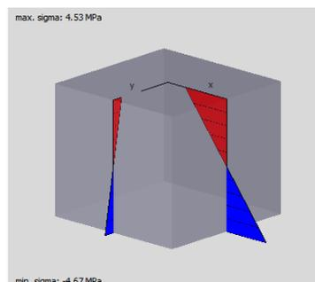
Figure 74: Concrete's stress-diagram
