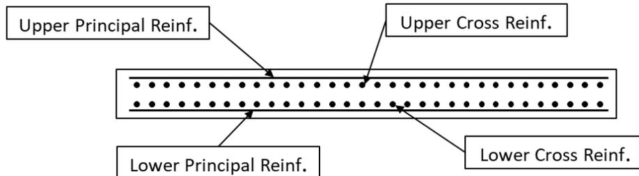
Figure 42: Cross-sectional view of generic slab
