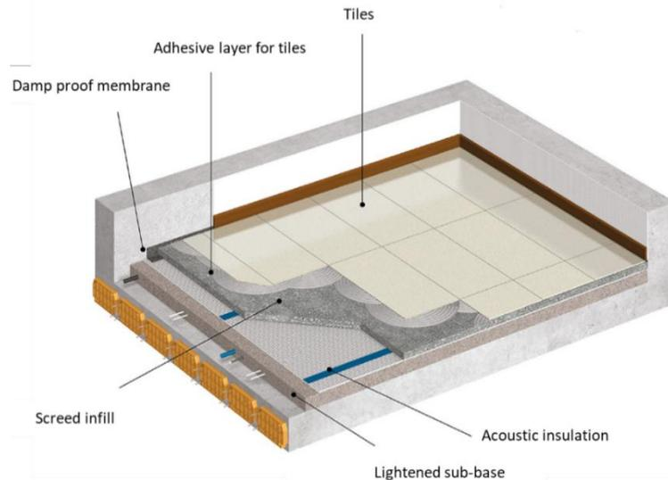
Figure 27: Paving scheme
