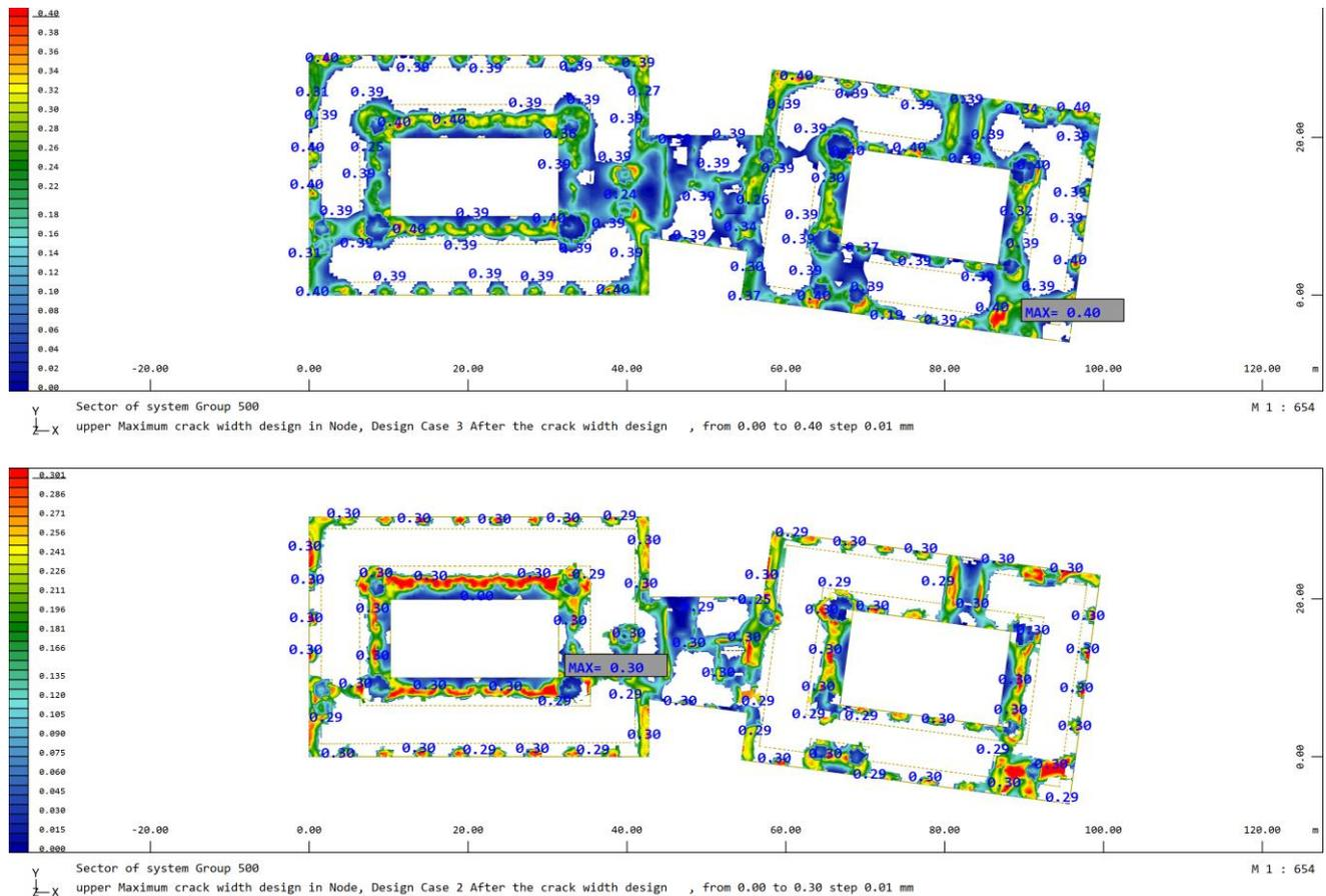
Figure 101: Cracks Expected in first floor slab
