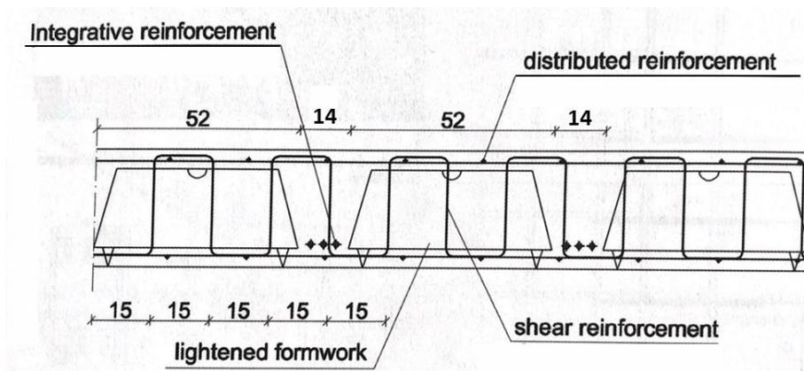
Figure 54: Positioning of shear reinforcement
