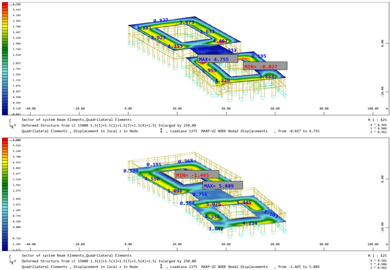
Figure 107: Vertical deformations in the slabs
