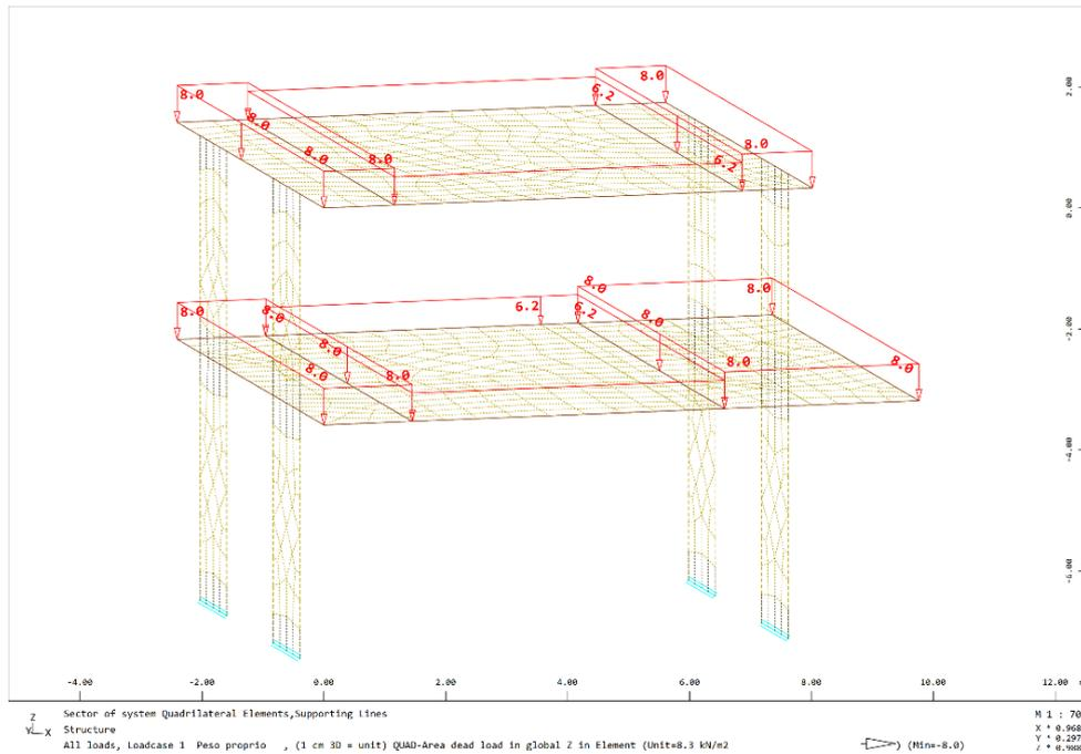
Figure 79: Self-weight of slabs - Alternative 3
