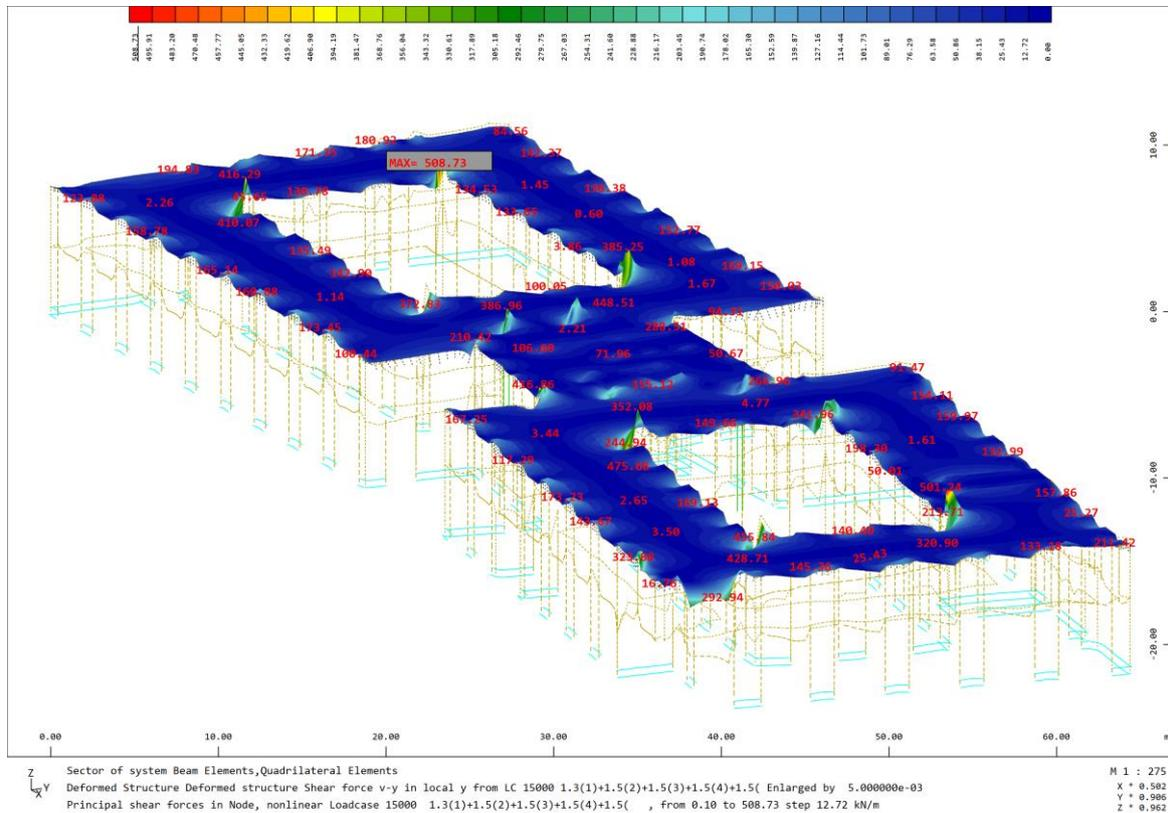
Figure 91: Shear Forces - Roof Slab
