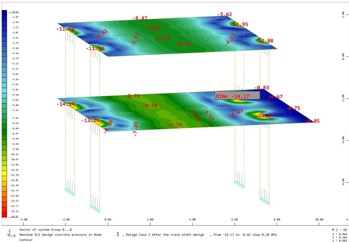
Figure 49: Compressive Stresses in long-term SLS
