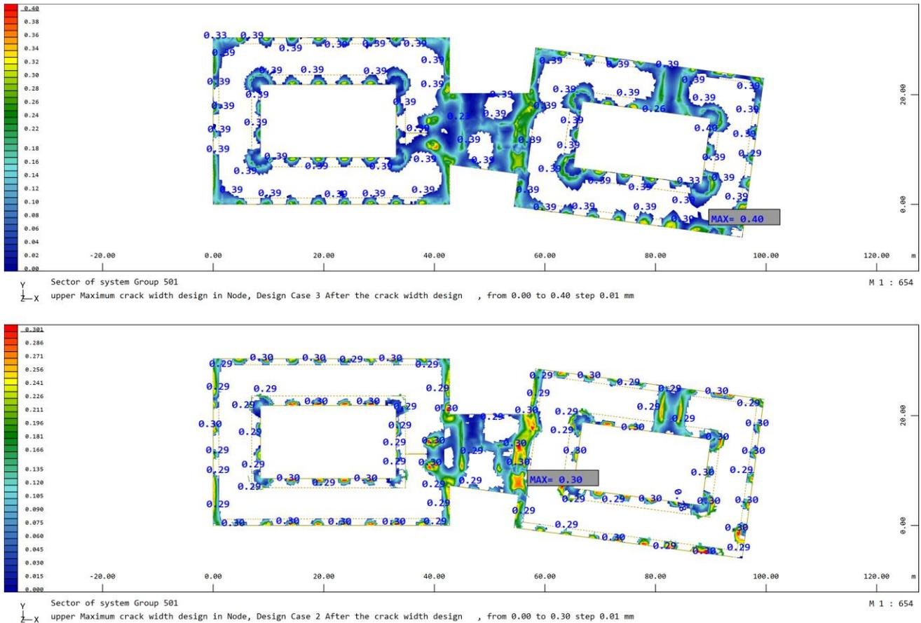
Figure 102: Cracks expected in roof slab
