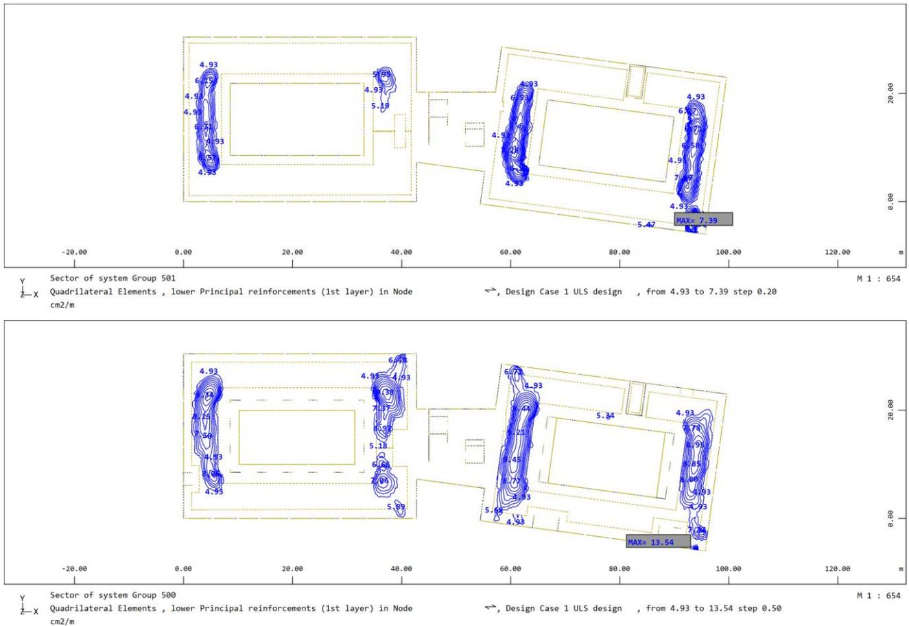
Figure 97: Lower principal reinforcement
