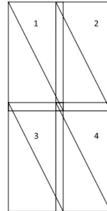
Figura 6 - arrangement of electro-welded meshes.
