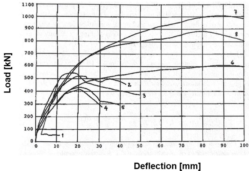
Figure 55: Study with 'hat' reinforcement
