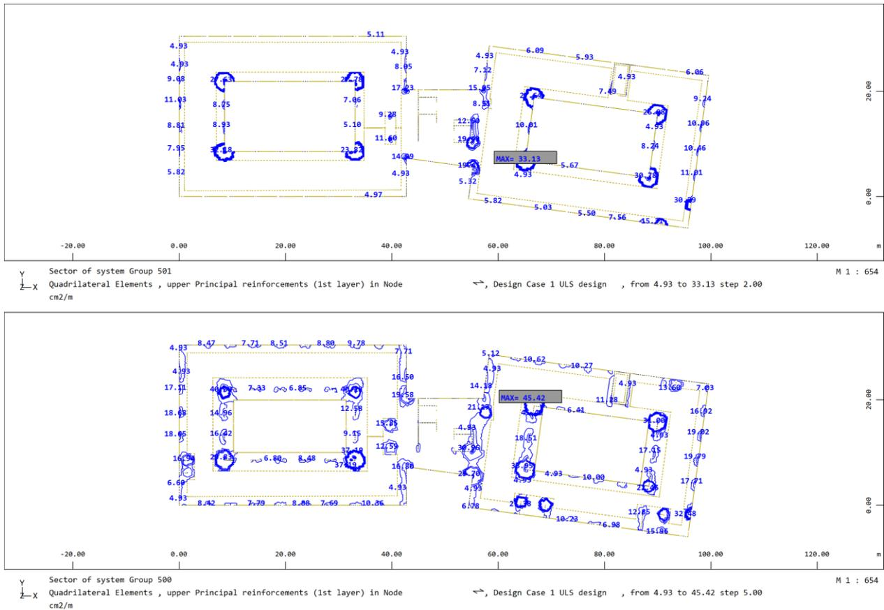
Figure 96: Upper principal Reinforcement
