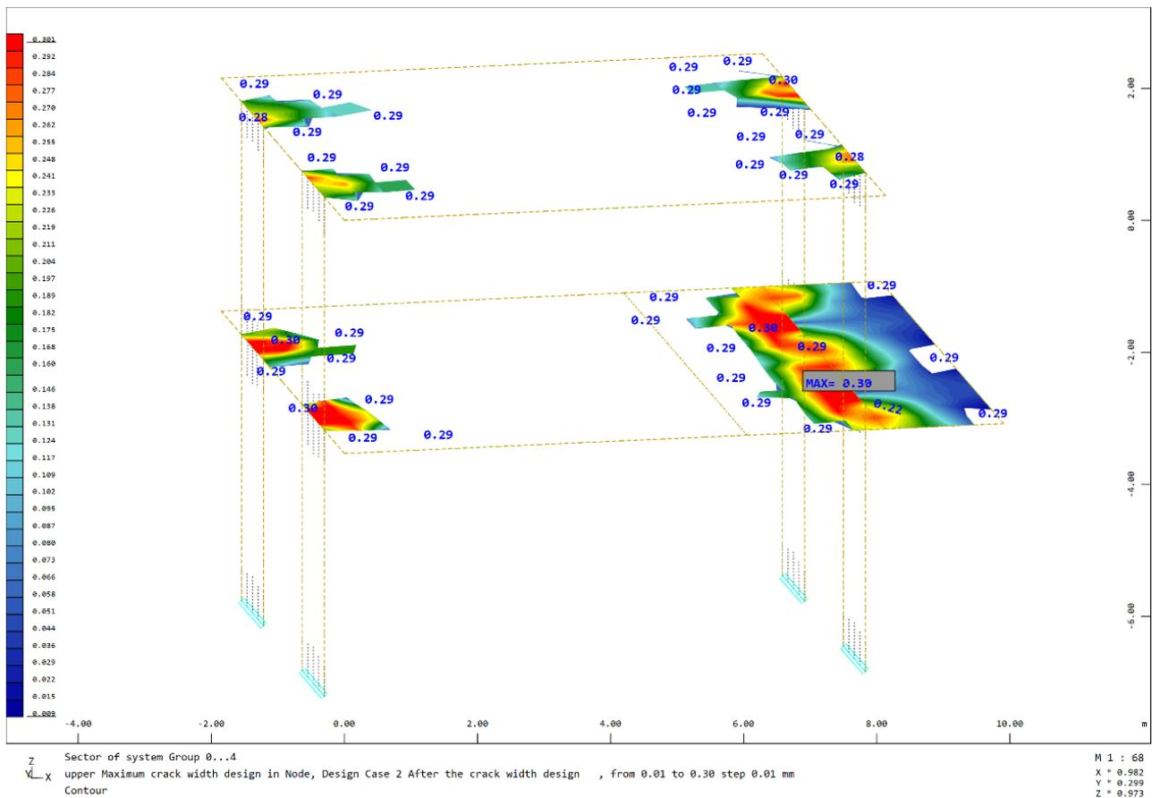
Figure 47: Expected cracks in quasi-permanent SLS
