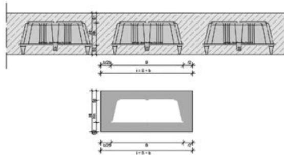
Figura 18 - section type - calculation of the reduction coefficients
