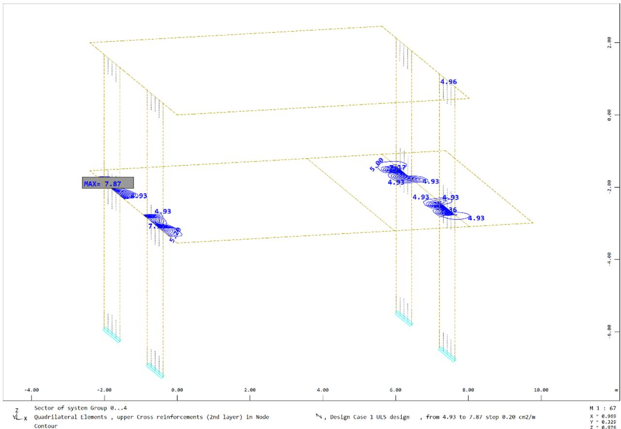
Figure 45: Upper cross reinforcement
