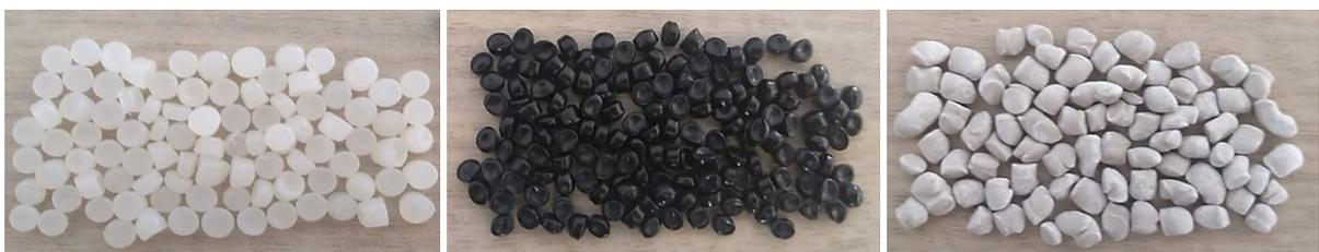
Figure 4. Left: HDPE pellets (before mix experiments). Middle left: Carbon black (35%) masterbatch pellets. Right: PE pellets with 82% chalk.
