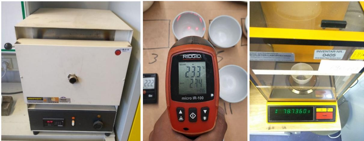
Figure 29. Left: oven for burn off experiments. Middle: temperature measurement of the sample cup. Right: measuring the mass of a sample.
