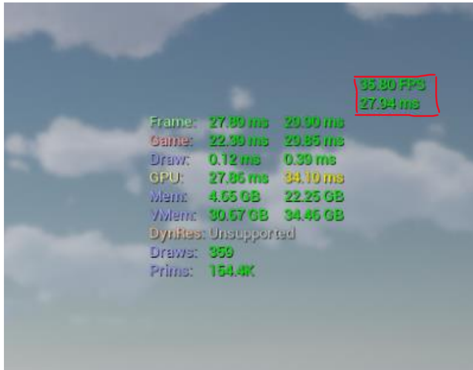
(Figure 47. Detail stats at run time. Top Right -> FPS and how much it takes to render one frame (red box). Below separate processes detailed individually. )
