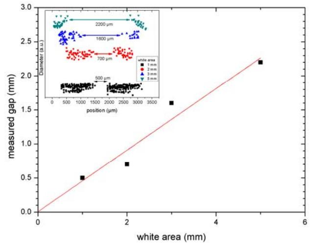
**Figure 10.** Measured gap between “hydrophobic” areas versus original width of white area from bitmap determined from Figure 9. Inset shows cross scan of the droplet diameters for the “hydrophobic” area. Arrows represent the measured hydrophilic gap.
