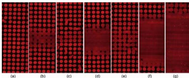
**Figure 3.** Fluorescent images of air plasma treated glass, inkjet printed with DEGDMA at 115 dpi for a selection of the DoE experiment. Letters correspond with the data in Table 2. At the centre of each image a single pixel wide plasma line was printed
