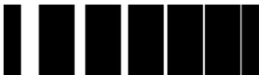
**Figure 2:** Bitmap used for experiment 3. Distance between treated (black) areas from left to right 5, 3, 2, 1, 0.5 and 0.3 mm. The black areas are respectively 5 (first and last) and 10 mm wide and 20 mm high
