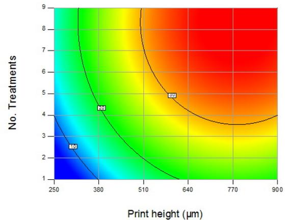
**Figure 6.** Contour plot of the width (in mm) for a single pixel wide atmospheric air plasma printed line versus print height and number of plasma treatments (Design of Experiments 2).
