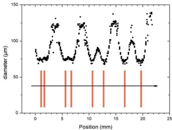
**Figure 8:** Droplet diameters of inkjet printed DEGDM for a cross scan of plasma printed (orange) lines). 200 ml/min  $N_2$  plasma with 20 ml/min saturated HMDSO+ $N_2$  plasma (print height 200  $\mu\text{m}$ , two treatments on glass)
