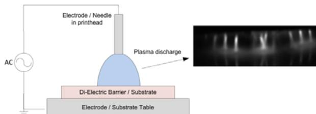
Figure 1. DBD plasma configuration for the Innophysics POD24  $\mu$ Plasma printhead. Photo on right shows multi-needle plasma discharge.
