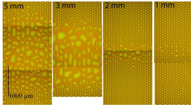
**Figure 9.** Microscope images of printed bitmap (figure 2) for respectively the 5,3,2,1 mm wide white area of figure 2. Treatment is 70x20 mm rectangle  $N_2$  plasma (5 treatments) followed by  $N_2$ +HMDSO plasma using figure 2 (one treatment) followed by inkjet printing of DEGDM at 315 dpi.
