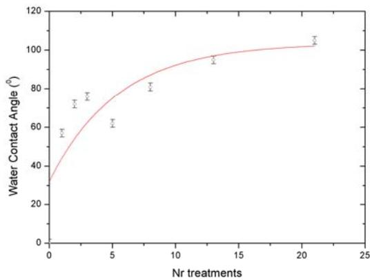
**Figure 7:** Water Contact Angle versus nr of treatments of a glass substrate treated with  $N_2$ + HMDSO plasma (flow:200 ml/min  $N_2$  and 20 ml/min HMDSO saturated  $N_2$ ) (red line is only shown to aid the eye of the reader)
