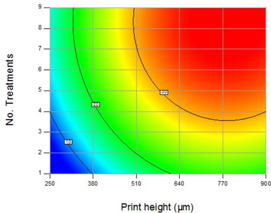
**Figure 4.** Contour plot of the width (in mm) for a single pixel wide atmospheric air plasma printed line versus print height and number of plasma treatments on a polycarbonate substrate (Design of Experiments 1).
